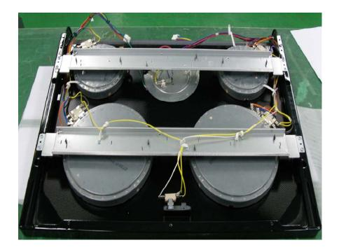
In either configuration if the cooking elements are not seated properly the cook top will not be assembled, installed or work properly.
