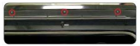
From here, the tech can either remove the rear covers and disconnect the wiring to the cook top and remove the assembly or just lift the front and pull out. There is in some cases enough slack in the wiring to do this.
