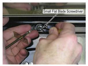
5. Install two screws that attach the sensor to the back of the oven liner.
