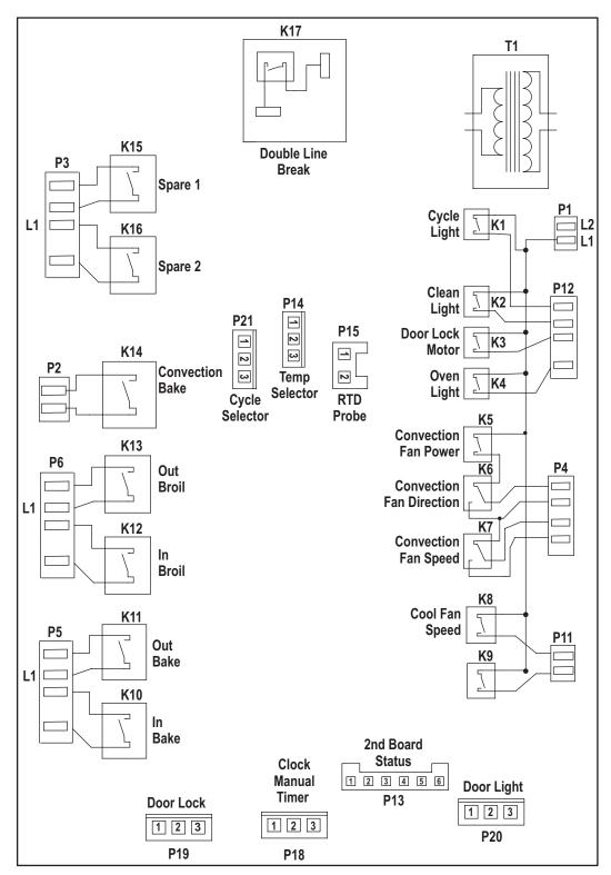
**Oven Control Board Schematic**
