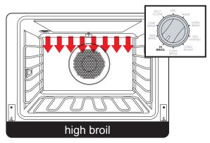
Heat radiates from both broil elements. The broil elements use approximately 240V and remain on constantly.
