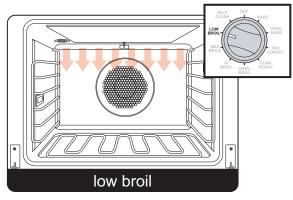
Heat radiates only from the inner broil element. The inner broil element uses approximately 240V and pulses on for 25 seconds and off for 35 seconds.
