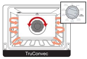
The convection element uses approximately 240V and pulses on for 53 seconds and off for 7 seconds. The convection fan remains in low speed, changing direction every 40 seconds.
