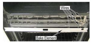
5. Remove the bake element from the oven
