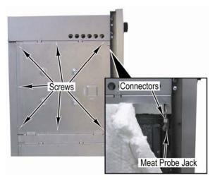
4. Lift the meat probe jack cover and remove the 5/8 inch nut that attaches the jack to the oven liner.
