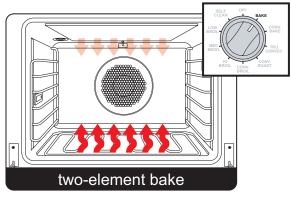
The bake elements use approximately 240V and the inner broil element cycles on and off at various times to maintain the set temperature. See the oven preheat chart for more information.
