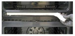
3. Remove the two screws that attach the bake element to the element shelf.
