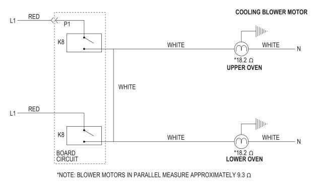
**Cooling Blower Motor Strip Circuit**
