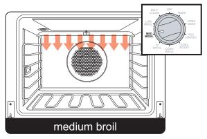
Heat radiates from both broil elements. The broil elements use approximately 240V and pulse on for 40 seconds and off for 15 seconds.
