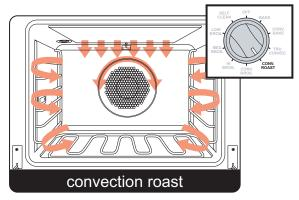
The convection element uses approximately 240V and pulses on for 40 seconds and off for 7 seconds. The convection fan remains in high speed, changing direction every 40 seconds. During the change in direction, the broil elements pulse on for approximately 2 seconds.
