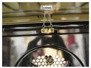
2. Pull the sensor from the liner until the sensor connector protrudes into the oven cavity.
