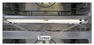
4. Slide the bake element partially out, mark and disconnect the four wires from the bake element.
