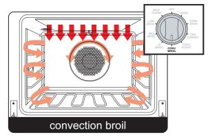
Heat radiates from both broil elements. The broil elements use approximately 240V and pulse on for 53 seconds and off for 7 seconds. Additionally, the convection fan cycles on for 40 seconds, cycles off for 7 seconds, and then cycles on in the opposite direction for 40 seconds. This cycle then repeats.
