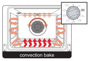
The convection element uses approximately 240V and cycles on and off at various times. The bake and broil elements use 240V and pulse on and off less frequently than the convection element. Additionally, the convection fan cycles on for 40 seconds, cycles off for 7 seconds, and then cycles on in the opposite direction for 40 seconds. This cycle then repeats.
