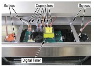
6. Remove two screws and mounting bracket from each side of the timer.
