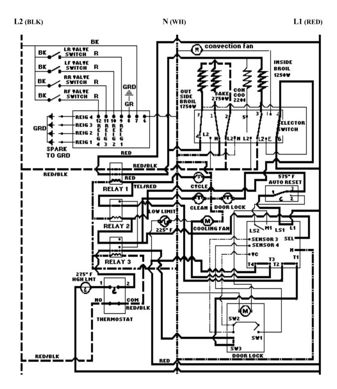
Auto Reset switches to 1-3 which turns Door Lock Indicator Light on and disables Door Lock Motor circuit.
