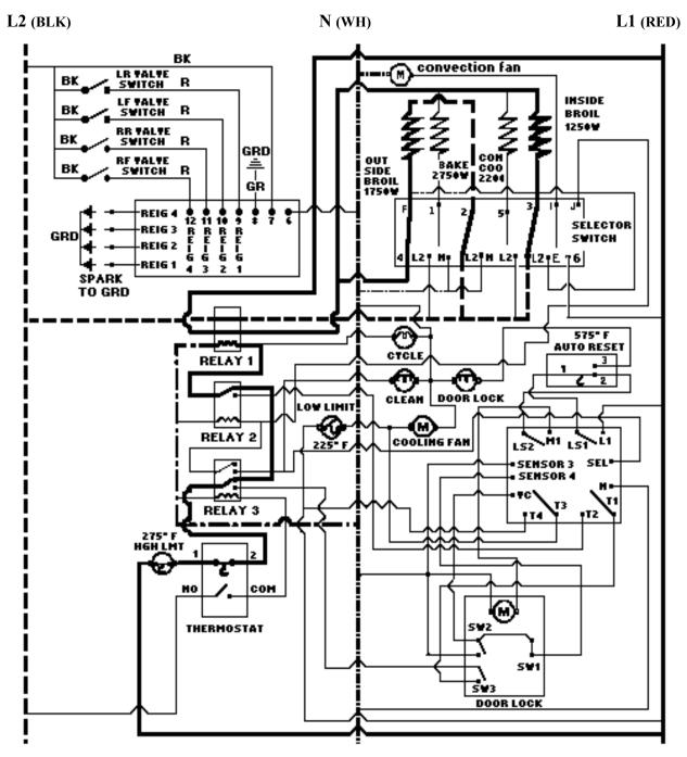
**Selector Maxi Broil** position closes Switches 4-F, 2-L2, and 3-L2. The Thermostat closes Switch Cy1-Cy2, which cycles with the oven temperature, powering Relay #1 and the Oven Cycle Light. When Relay #1 closes, it powers the inside Broil Element at 208v / 240v and the Outside Broil Element at 208v / 240v.
