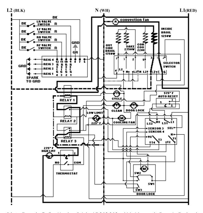
**Selector Convection Broil** position closes Switches 4-F, 2-L2, 3-L2, and 6-1. 6-1 powers the Convection Fan through L1 at 120v. The Thermostat closes Switch Cy1-Cy2, which cycles the Oven temperature, powering Relay #1 and the Oven Cycle Light. When Relay # 2 closes it powers the inside Broil Element at 208v / 240v and the outside Broil Element at 208v / 240v.
