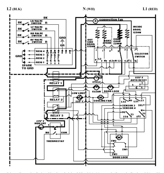
**Selector Convection Cook** position closes Switches 5-L2 and 6-1. 6-1 powers the Convection Fan through L1- at 120v. The Thermostat closes Switch Cy1-Cy2, which cycles with the Oven temperature, powering Relay #! and the Oven Cycle Light. When Relay #1 closes, it powers the Convection Element at 208v/240v.
