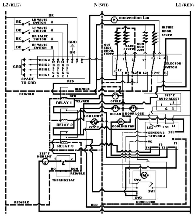
10 seconds after the signal to Sensor #3, Switch LS2-M1 is opened, stopping the door lock motion and Switches T1- T2, and T3-T4 which switches Relay #1, powering the Cooling Fan, which closes Relay #1 powering the inside and outside Broil Elements to 208v /240v and the Bake Element to 120v.
