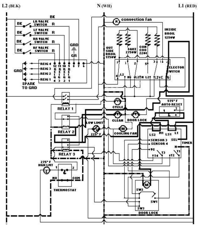
Auto Reset Switches 1-2 closed allowing the Door Lock Motor to operate and turning the Door Lock Light off. The Door Lock Motor operates until 2 seconds after Sensor 4 is signaled be VC that the Door Lock SW1 has been closed mechanically by the Door Lock bolt. The Door Lock / Timer switches LS2-M1 and LS1-L1 open and the Timer resets.
