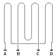
**Convection Element:** "A" to "B" 26 ohms "A" to "B" 240vac during convection cook
