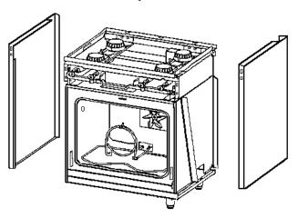
Remove the 6 screws along the upper frame above the door that hold the burner box assembly to the oven body. Lift the front of the burner box high enough to gain access to the **self clean lock** and associated components (High Limit Switch and Cooling Fan Switch ). Use a block, approximately 6" high, to hold the burner box in place while working on the lock.
