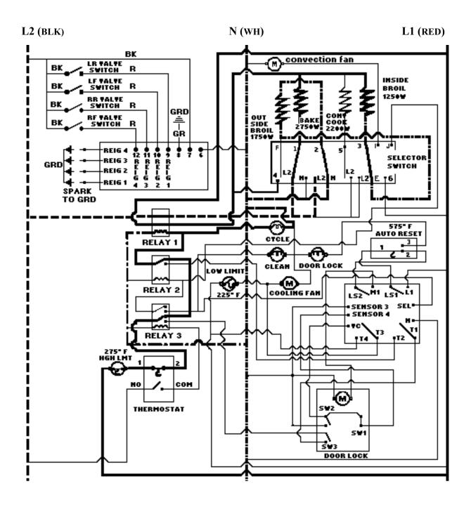
**Selector Bake** position closes Switches 1-L2, 2-N, and 3-E. The Thermostat closes Switches Cy1-Cy2, which cycles with the oven temperature powering Relay 1 and the Oven cycle light. When Relay 1 closes, it powers the Bake Element at 208v/240v, and with the Broil Element in series across a 120v circuit, it powers the inside Broil Element at 70v and the outside Broil Element at 50v.
