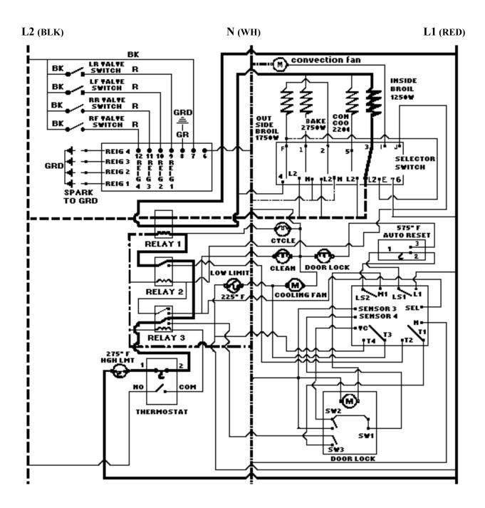
**Selector Mini Broil** position closes Switches 3-L2. The Thermostat closes Switch Cy1-Cy2, powering Relay #1 and the Oven Cycle Light. When Relay #1 closes, it powers the inside Broil Element at 208v/240v.
