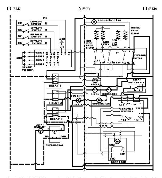
Timer Switches T3-T4, T1-T2 open, turning off the Cooling Fan, which will then be powered at 120v by the Fan Limit Switch when needed, and opening the circuit to Relay #1 which disables the Heating Elements. Switch LS2-M1 closes to power the Door Lock Motor.
