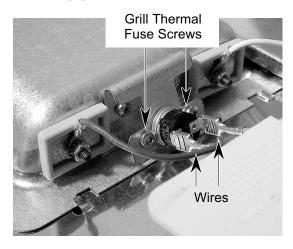
b) Remove the two thermal fuse mounting screws.
