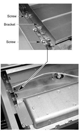
c) Slide the grill element assembly to the left and release the slots from the locking tabs. NOTE: It may take a moderate amount of force to do this.
