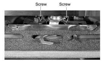
5. Remove the lower oven door latch assembly and disconnect the wires from the two switches and the solenoid terminals.
