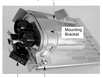
High Voltage Clamp Screw Rectifier
