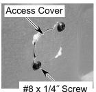
REASSEMBLY NOTE: When you install the new jack, be sure to place the star washer from the old jack on the threaded end of the new one. After you have installed the jack, mount the access cover with two #8 x 1/4" screws.
