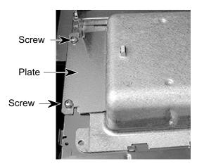
b) Remove the two T-10 torx screws from the bracket over the left end of the grill element assembly and raise the bracket slightly.
