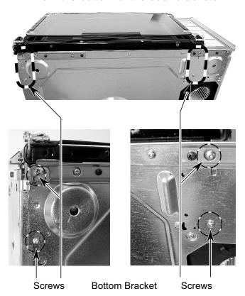
8. Pull the brackets out of the oven slots and remove the door assembly from the microwave.
