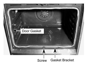
3. Pull the ends of the gasket out of the liner holes.
