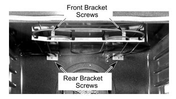
4. Carefully pull the element forward so that the terminal connectors are through the oven liner holes, and disconnect the wires from the terminals.
