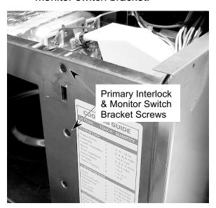
d) Disconnect the wires from the primary interlock and monitor switch terminals.
