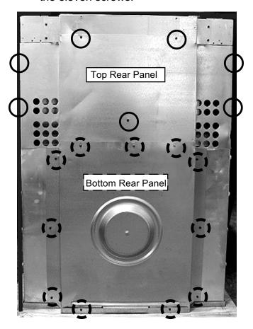
4. To remove the top rear panel, remove the remaining seven screws.
