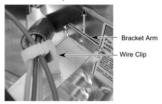
d) Lift the arm out of the rear panel track, and remove the mounting bracket assembly.
