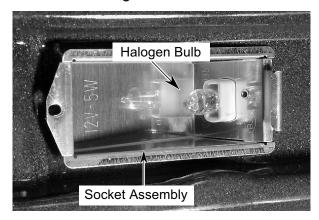
Pull the halogen socket assembly out of the oven liner and cut the wires near the socket terminals.
