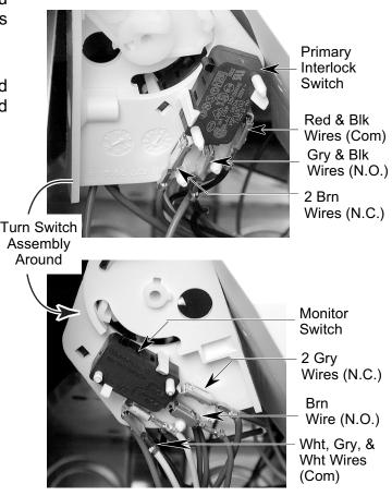
e) Unclip and remove the primary interlock and monitor switches from the bracket.
