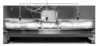
d) Carefully move the upper and lower sections of the insulation blanket out of the way so that you can access the hidden bake element and its mounting bracket. e) Remove the four mounting bracket screws and the two hidden bake element bracket screws.
