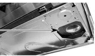
d) Remove the T-10 torx screws from the fan motor and remove the motor from the housing.
