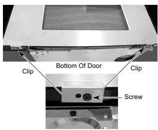
**CAUTION:** When you remove the front door glass and handle in the next step, be careful when you remove the two screws that hold the assembly together. Hold the door open while you remove the screws; otherwise the door will spring closed. Also, be careful not to drop the glass and handle assembly when you remove the screws.
