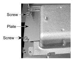
b) Remove the two T-10 torx screws from the bracket over the left end of the grill element assembly and raise the bracket.
