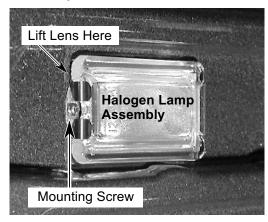
5. Pull the halogen bulb out of the socket.
