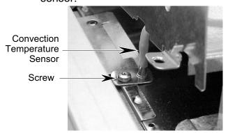
d) Remove the two sensor wires from the harness.
