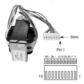
Refer to page 2-4 for the procedure for servicing the low voltage transformer.
