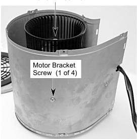
8. Remove the mounting nut from each of the blower wheels and remove the wheels from the blower motor.
