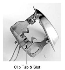
6. Remove the two screws from the socket and remove the socket from the holder.
