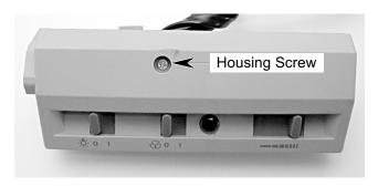
Separate the two sections by rotating the slide switch section away from the housing and unsnapping the two tabs from their slots.
