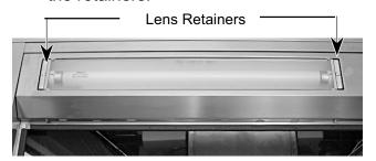
Slide the fluorescent lamp lens to either end of the holder and remove it from the holder tabs.
