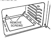
5. Remove the heat shield from the oven .
