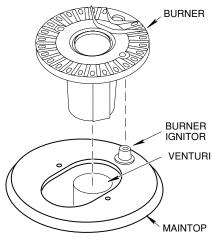
5. Push the front of the maintop to the right while lifting the right corner and unclip it, then push to the left and unclip the left corner. Lift the maintop and prop it up.
