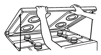
2. Adjust the air shutter openings, as needed. Close the air shutter to decrease the amount of air to the flame. Open the air shutter to increase the amount of air to the flame.
