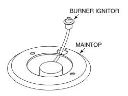
9. Slide the maintop to the right so that the left hinge pin is free of the hinge bracket, (see the inset), and then to the left so that the right hinge pin is free of its bracket, then set the maintop with the burner ignitors on top of the range. CAUTION: Be careful not to pull on the spark ignitor wires or you will pull them out of the ignitors.
