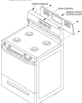
Without disconnecting any wires, remove the mounting screws from the electronic oven control and remove it from the back of the console.
