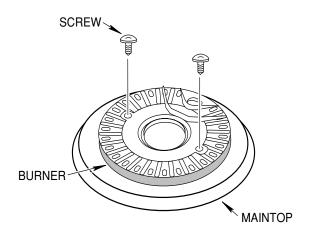
3. Lift each burner off the venturi and burner ignitor.
