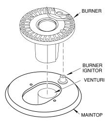
4. Push the front of the maintop to the right while lifting the right corner and unclip it, then push to the left and unclip the left corner. Lift the front of the maintop and prop it up.
