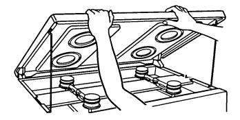
4. Slide the maintop to the left so that the hinge pin is free of the right hinge bracket, (see the inset), and to the right so that it is free of the left bracket, then remove the maintop.
