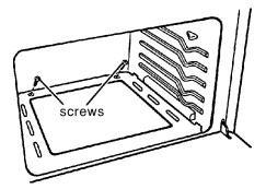
3. Remove the screws from the heat shield over the oven burner and remove the shield.
