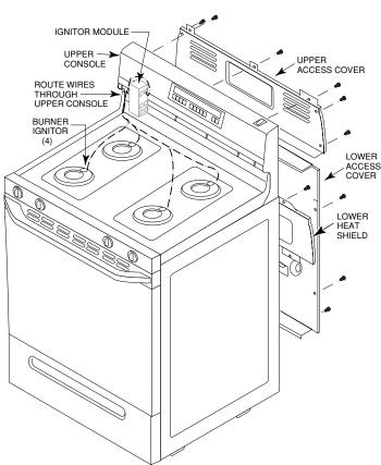
8. Unplug the burner ignitor wires from the ignitor module, pull them through the back of the upper console to the front, and remove them from the maintop.
