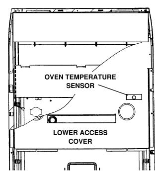
4. Disconnect the wire harness from the old oven temperature sensor and remove the sensor from the range.
