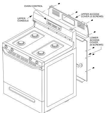
4. Remove the oven control and green ground wire (if present) from the upper console. It is not necessary to disconnect the wires from the control.
