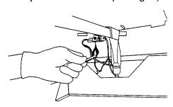
Turn the oven control to 350°F. The oven burner should light in 20- to 40-seconds (the delay is due to the time it takes for the gas valve to open and the gas to flow to the burner).
