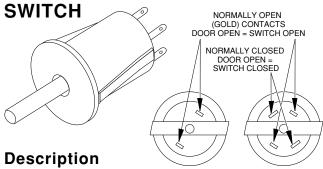
The automatic oven light switch contacts are normally open when the oven door is closed and the plunger is pushed in. When the door opens, the plunger is pushed out, the contacts close, and 120-volts is applied to the light, which then turns on.
