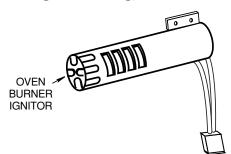
Steady State Current = 2.5 TO 3.0 Amps @ 115  $\pm$ 1 VAC @ 75°F  $\pm$ 10° Ambient.
