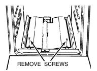
6. Remove the front and back mounting screws from the oven burner.
