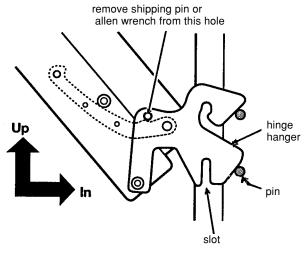
2. Remove the shipping pins and close the door.
