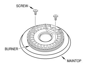
4. Lift each burner off the venturi and burner ignitor.
