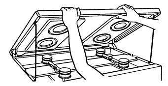
3. With the burner control knobs at OFF, use a match, and light both of the pilot lights.
