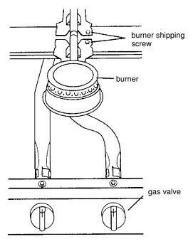
4. Removing one orifice spud at a time, use a <sup>3</sup>/<sub>8</sub>"combination wrench, and replace the natural gas orifice spuds with the L.P. gas orifice spuds. NOTE: When you are finished, place the natural gas orifice spuds in a plastic bag, and store them in a safe place for possible future use. Also, keep the literature that was supplied with the orifice spuds, in the same bag.
