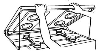
4. If installed, remove the shipping screw from the burner, then lift and unhook the burner from the burner bracket, and remove it from the range.
