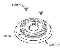
Lift the defective burner off the venturi and replace it with a new one, then reassemble the range.
