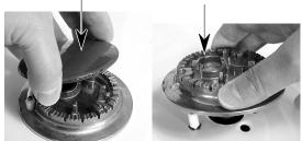
4. Remove the mounting screw from each of the four burners.
