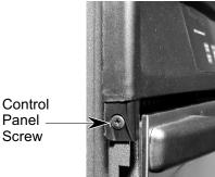
6. To remove the oven control panel, pull it out at the bottom, and lift and unhook it from the oven cabinet support at the top.
