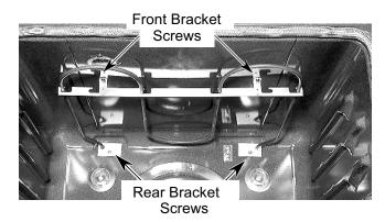
4. Carefully pull the element forward so that the terminal connectors are through the oven liner holes, and disconnect the wires from the terminals.
