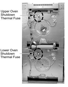
4. Disconnect the wires from the thermal fuse terminals.
