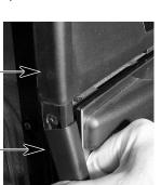
5. Remove the screws from the oven control panel.
