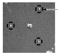
Convection Fan Motor Front Screw (1 of 3)
