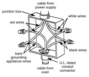
Separate Grounding Conductors To White (Neutral) & Bare Wires
