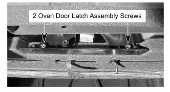
e) Remove the lower oven door latch assembly and disconnect the wires from the two switches and the solenoid terminals.
