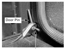
Door Pin Into Hinge Hanger Hole
