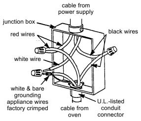
Crimped Grounding Conductors To White (Neutral) Wire
