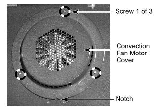
Use a 10 mm (7/16") socket and remove the hex nut from the convection fan. NOTE: The nut has a left-rotation thread for removal.
