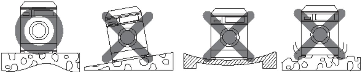
④ Adjust leveling with the leveling legs.
