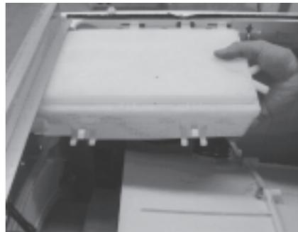
3. Remove and separate inlet bellows hose.
