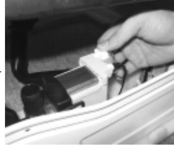
4. Remove pump in the direction of arrow.
