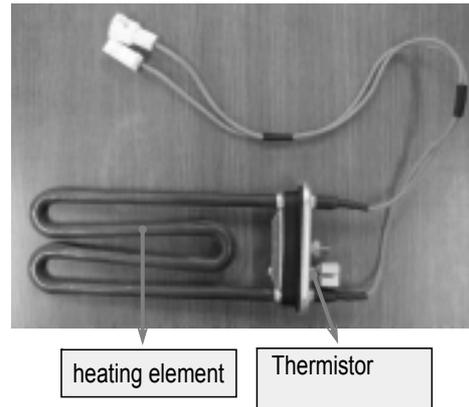
Temp. Fuse of Washing Heater 363°F (184° C CUTOFF TYPE)
