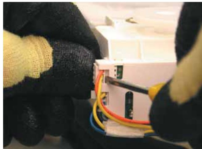
2. Remove the 2 Phillips-head screws that attach the motor and gasket inlet hose clip to the dispenser tank. (See **Dispenser Assembly**.)
