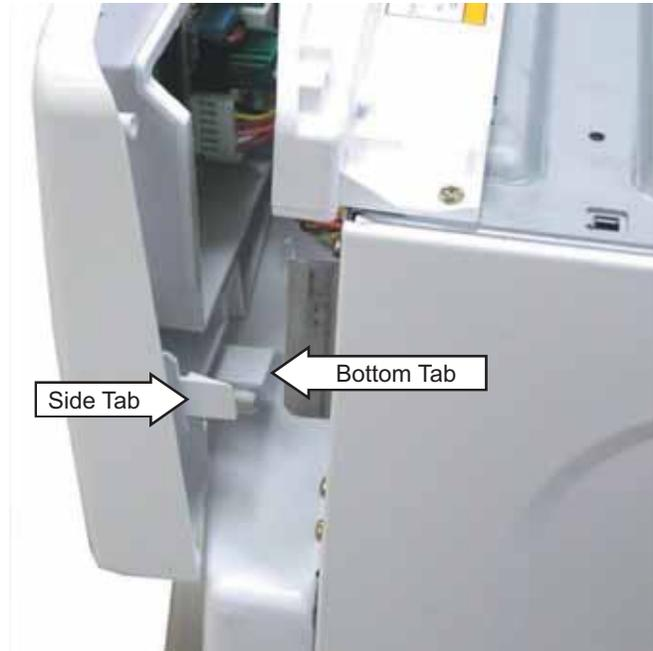
6. Lift the top edge of the panel to disengage the 3 tabs that hold the top of the panel in place.
