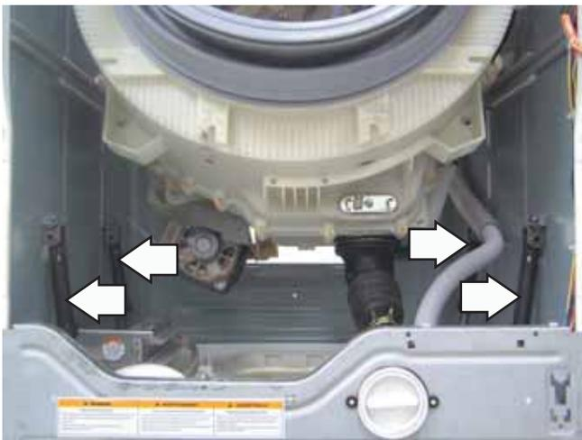
18. Lift the outer tub assembly up, then release the 2 suspension springs from the slotted plastic inserts in the cabinet top braces.
