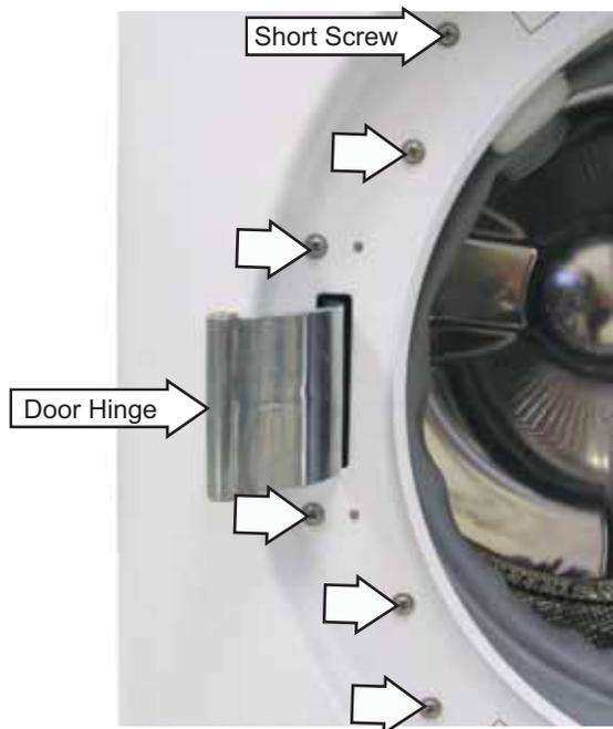
**Caution:** When reinstalling the door hinge, be sure to use the short screw on the top. Damage to the dispenser inlet may result if the wrong screw length is used.
