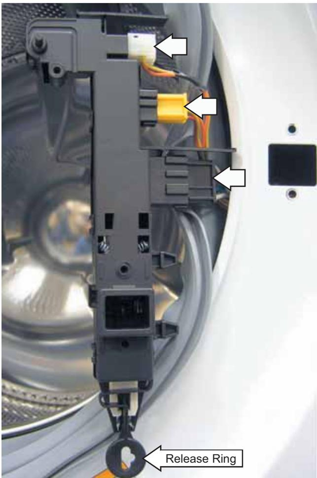
**Note:** The door latch is solenoid activated. It can remain locked after power is removed.
