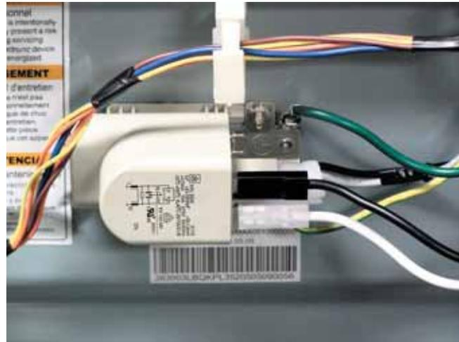
4. Remove the 2 (7-mm) hex-head screws that hold the filter to the frame.
