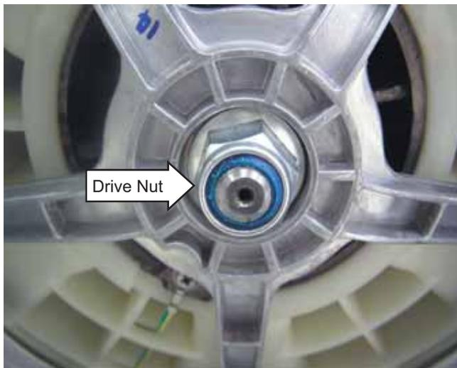
**Caution:** The nylon locking material used inside the drive nut will be damaged upon removal. Use replacement drive nut (Part # WH02X10211) when reinstalling the tub drive pulley. Use a torque wrench to tighten the 24-mm hex nut to 44 ft. lbs of torque.
