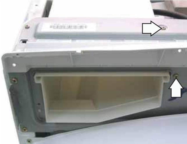
9. Remove the 8 Phillips-head screws that attach the control rear cover and the front bracket.
