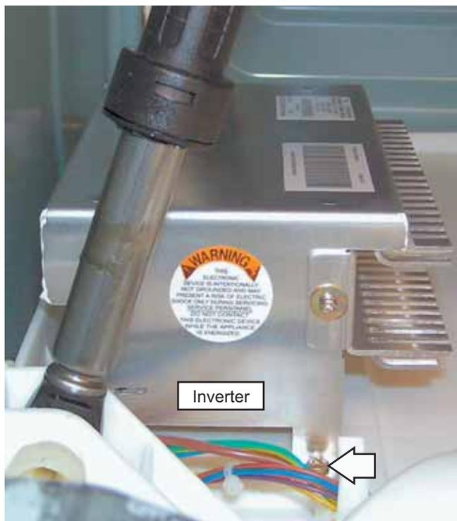
8. Slide the inverter rearward to clear the guides that hold the rear of the inverter to the chassis.
