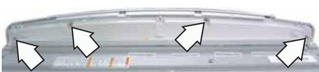
5. From inside the cabinet, lift and push forward to release the bottom tab from the front bracket.
