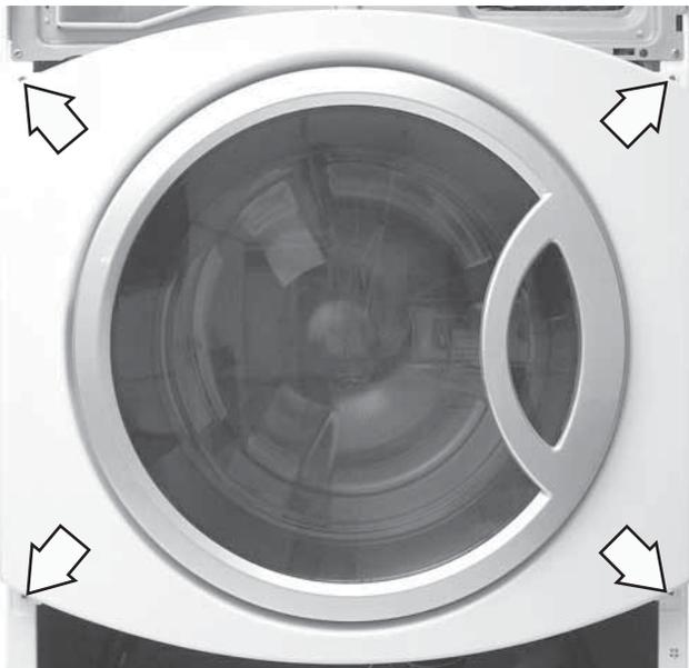
7. Lift up then remove the front panel from the 2 hooks.
