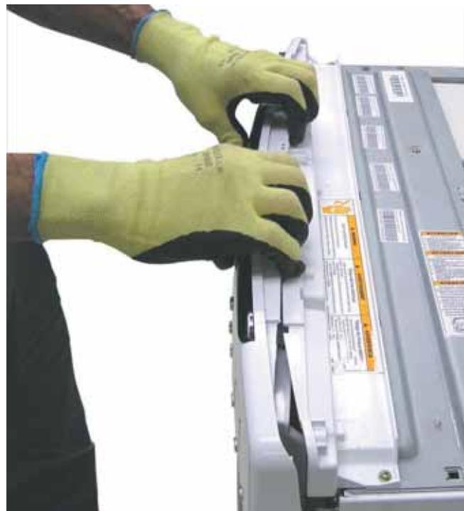
7. Push the control panel towards the left, then release the side tab.
