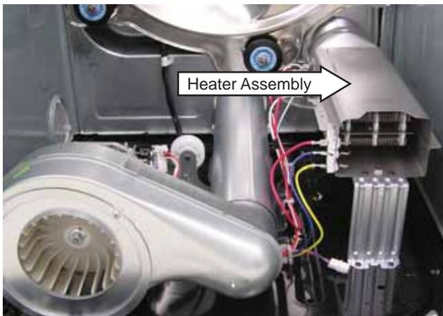
To remove the heater assembly:
