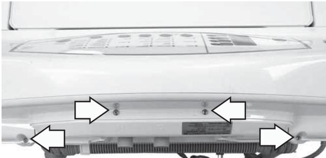
2. Place a towel over the lid of the washer to prevent scratches to the surface. Lift each corner of the backsplash vertically while pulling back to disengage the 2 tabs. Roll the backsplash forward so it rests on top of the washer.
