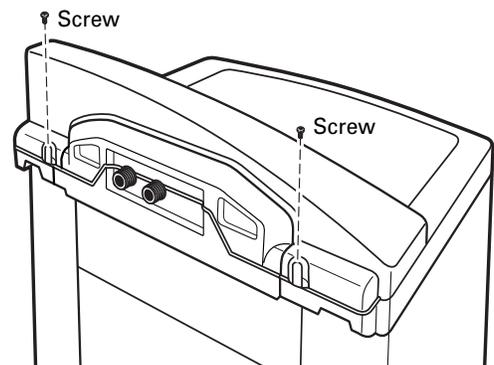
20. Secure the new washer backsplash to the rear cover using the 2 Phillips head screws removed earlier.
