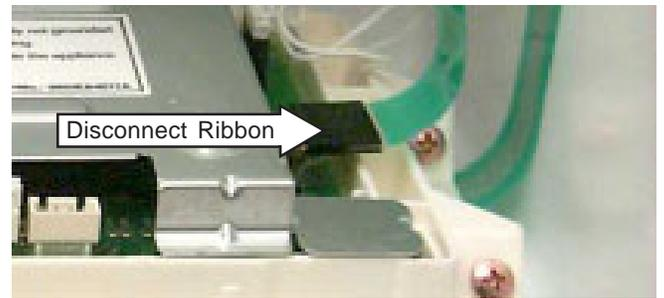
3. Remove the 4 Phillips head screws (2 on each side) that hold the main control board and LCD touch screen assembly in place. Remove the assembly.
