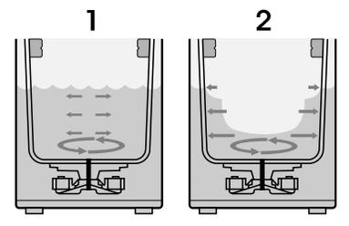
As water passes through the fabric, its natural cleansing action washes away dirt without damaging or tangling the fabric.
