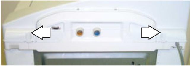
2. Place a towel over the lid of the washer to prevent scratches to the surface. Gently lift each corner of the backsplash, then roll it forward so it rests on top of the washer.
