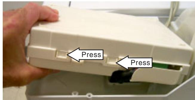
4. Disconnect the wiring from the inverter board. Remove the inverter.
