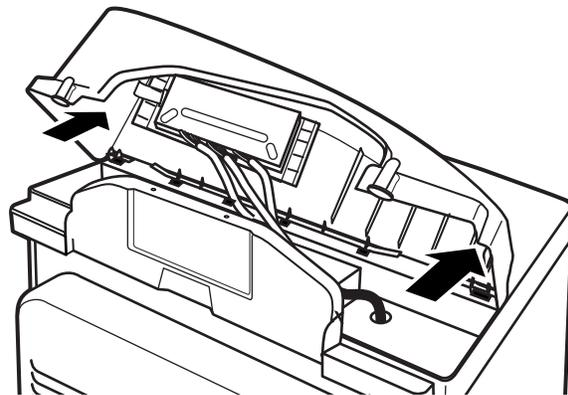
14. Connect the dryer control board to the new backsplash by sliding the ribbon connector on the new backsplash onto the metal pins on the control board and pushing in. Make sure the ribbon is not twisted before inserting the connector.
