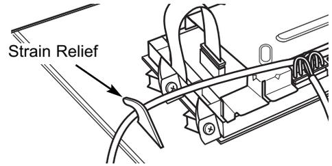
19. Connect the washer control board to the new backsplash by sliding the ribbon connector on the new backsplash onto the metal pins on the control board and pushing in. Make sure the ribbon is not twisted before inserting the connector.
