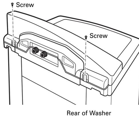
4. Remove the 2 Phillips head screws holding the backsplash to the rear cover. Remove the backsplash from the rear cover.
