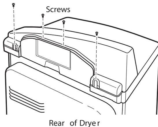
18. Attach the washer control board to the new backsplash by replacing the 4 Phillips head screws removed from the washer control board earlier.
