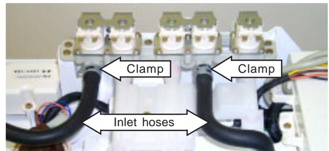
5. Remove the 3 Phillips head screws that hold the water valve assembly in place and the 2 Phillips head screws that hold the water distribution pipe in place.
