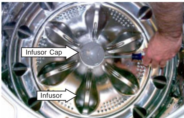
4. Remove the 10-mm hex-head screw that holds the infusor in place with a socket or Phillips head screwdriver (turn screw counterclockwise to remove).
