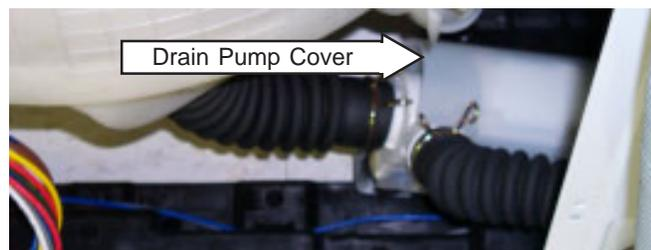
4. Remove the drain hoses from the pump:
