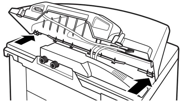
23. Secure the new backsplash to the washer using the 2 Phillips head screws removed earlier.
