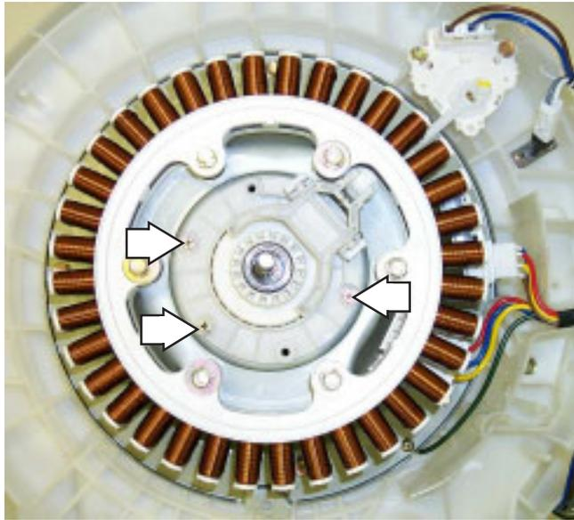
3. Remove the clutch coupler assembly.
