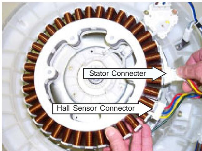
**Note:** When reassembling, be sure to put the motor and Hall sensor wires back in the wiring guard away from the motor.
