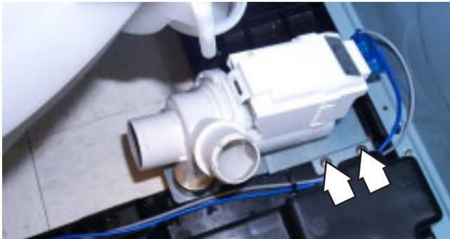
6. Disconnect the drain pump wires.
