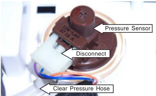
The pressure sensor wires (purple, orange, and blue) are connected at pins 1, 3, and 4 at the 4-pin red connector on the inverter board. (See ***Inverter and Main Board Pin Connectors***).
