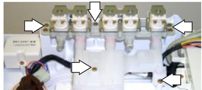
6. Remove the water valve assembly and distribution pipe.
