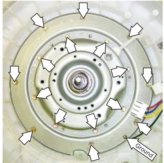
4. Remove the bearing housing assembly.
