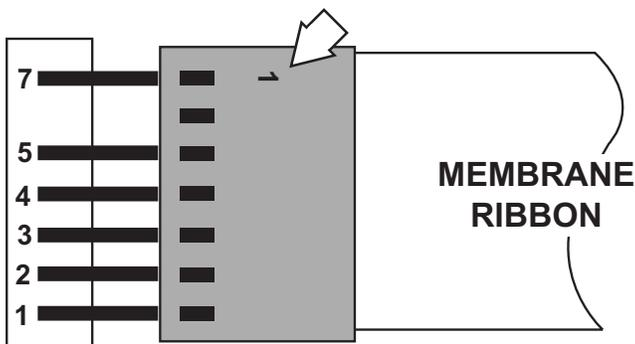
**Note:** The number (1) molded on the membrane connector is not a pin reference number.
