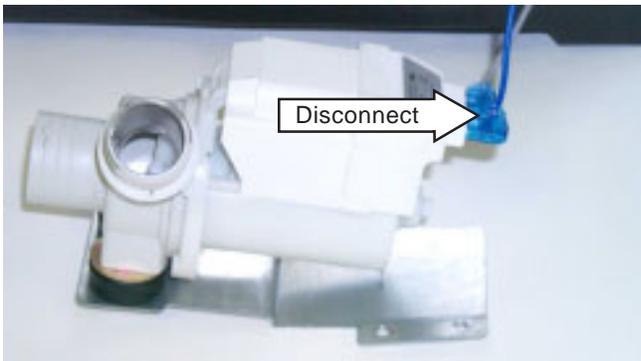
7. Remove the 2 Phillips head screws that hold the drain pump to the mounting plate. Remove the drain pump.
