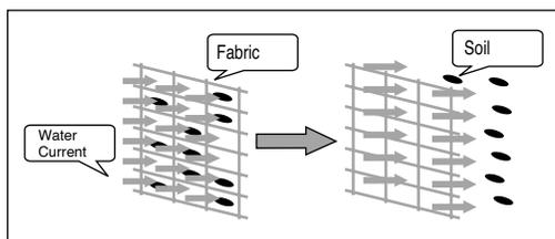
After several seconds of clockwise spinning, the basket slows down and stops. The wash water pools back into the wash basket. The wash basket starts spinning in the counterclockwise direction creating the same cleaning action. The washer will change direction (up to four times) before going to the next cycle.
