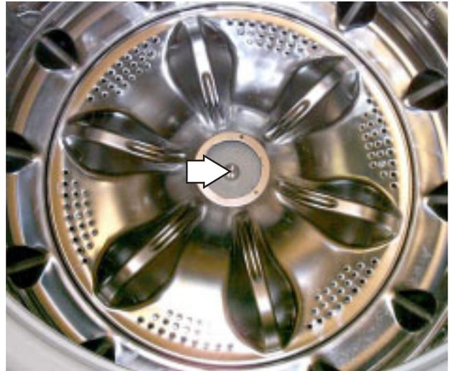
5. Pull the infusor up and out. **WARNING:** The inner edge can be sharp. Wear Kevlar gloves or equivalent protection.
