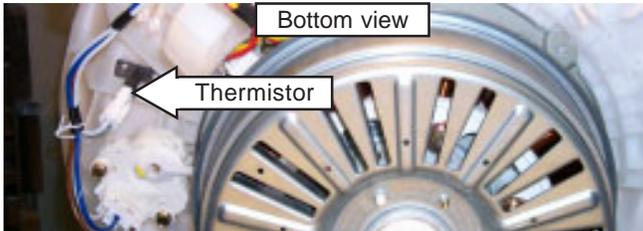
To determine the temperature of the incoming water, the washer control measures the difference between the voltage sent and the voltage returned from the water temperature sensor. The washer control then makes temperature adjustments accordingly.
