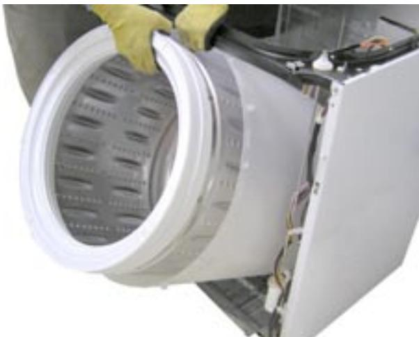
18. Remove the tub assembly from the cabinet and place it on a protected surface.
