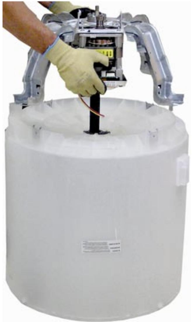
11. Place the platform upright on a protected surface and remove the tub bearing washer from the tube.
