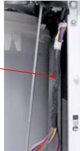
If the fuse is open, agitate, spin, and mode shifting does not occur. Check the fuse connections and wiring harness.
