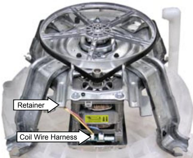
6. Run the belt off the drive pulley and remove the 3/4-in. pulley nut.
