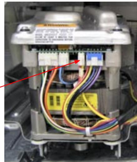
**Note:** The mode shift coil connects to C7 connector on inverter/motor assembly. Unplug C7 connector and check continuity. Mode shift coil resistance value is approximately  $98\Omega$  @ room temperature (77° F).
