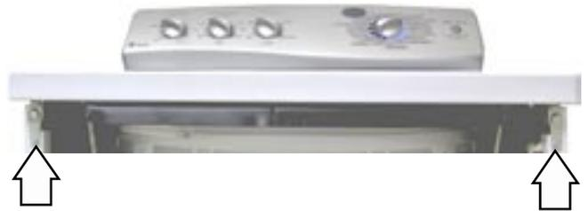
4. Pull the top cover toward you while lifting up the front edge to release the side catches. Slide the top cover to the left to release from the 3 tabs.
