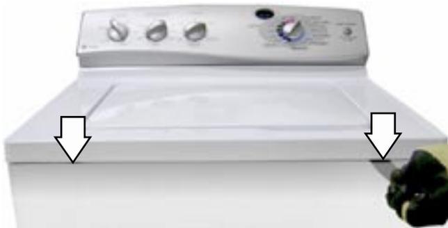
3. Rotate the front panel forward and lift off the bottom tabs.
