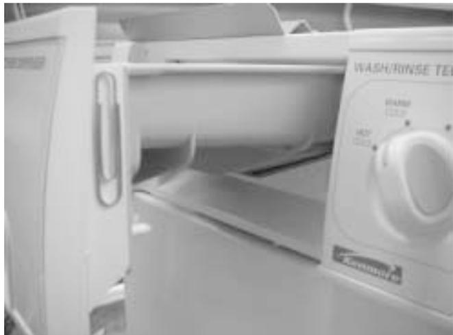
The reed switch connector can be accessed, with the top removed. Separate the connector and the reed switch pins. The dispenser door open is NO continuity. The dispenser door closed is continuity.
