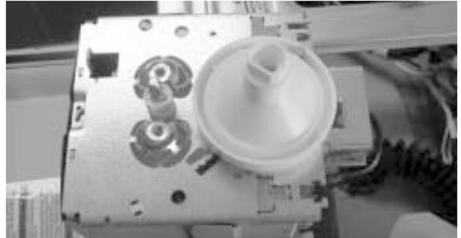
All other selector knobs are D-shaped and can be removed by pulling straight out.
