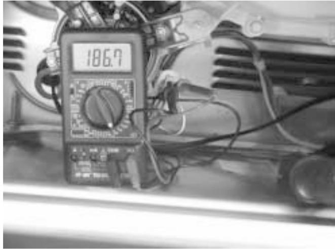
With volt/ohmmeter probes attached to the right and center leads, the reading should approximate the one in the picture. With a required resistance of 184 ohms, this reading is within the acceptable range. The information is provided in the schematic. Remember to access the tachogenerator leads from the front.
