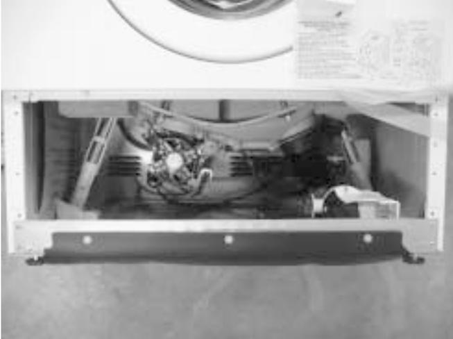
With the front panel removed, and the motor connector exposed, you can check the motor windings. They are color coded in the schematic as black, blue, and red.
