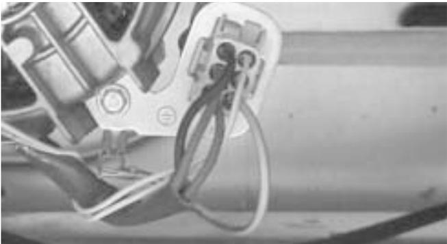
**Black is #1 Winding, Blue is #2 Winding, Red is #3 Winding**
