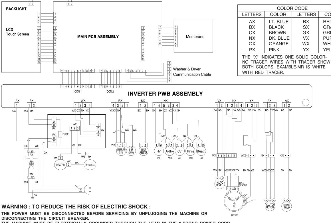
THE MACHINE MUST BE ELECTRICALLY GROUNDED THROUGH THE LEAD IN THE 3-PRONG POWER CORD THE CORD MUST BE PLUGGED INTO A APPLIANCE OUTLET THAT HAS BEEN PROPERLY INSTALLED. IF LOCAL CODES REQUIRE AN ADDITIONAL GROUND CONNECTION, USE A 15 GAUGE OR LARGER WIRE TO CONNECT THE WASHER CABINET TO AN ESTABLISHED GROUND. IN ALL CASES, THE GROUNDING METHOD MUST COMPLY WITH ALL LOCAL ELECTRICAL CODES AND ORDINANCES.
