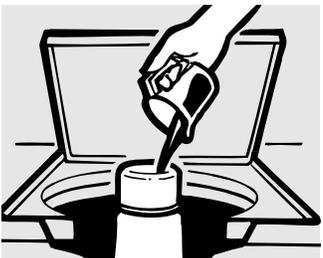
**The fabric softener dispenser** automatically releases liquid fabric softener at the proper time during the cycle.
