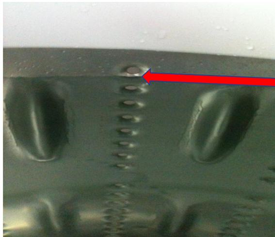
Approximately between 1st and 2nd sidewall hole from the top. (When this level is reached, water fill will stop and drain pump will come on.)
