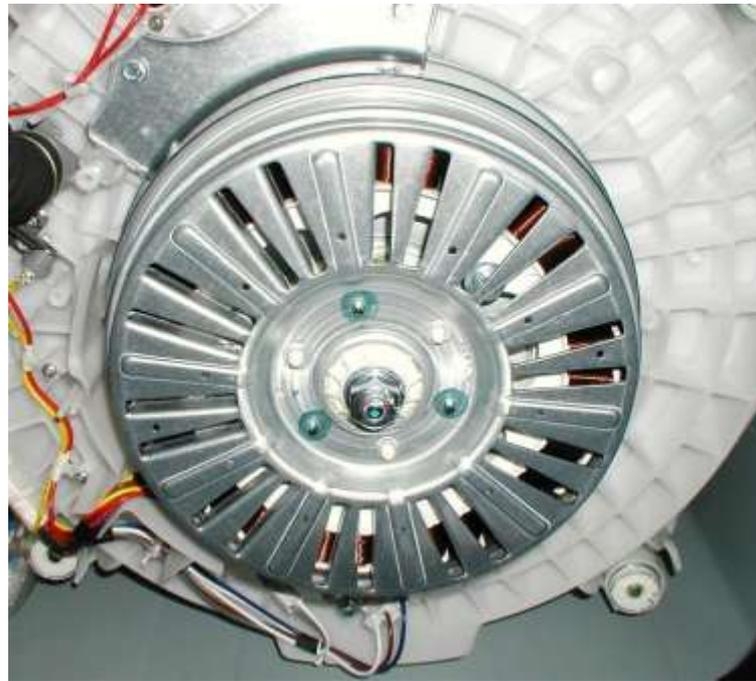
**Warning** : The rotor is not grounded & is moving when the motor is energized. Unplug the washer before servicing.
