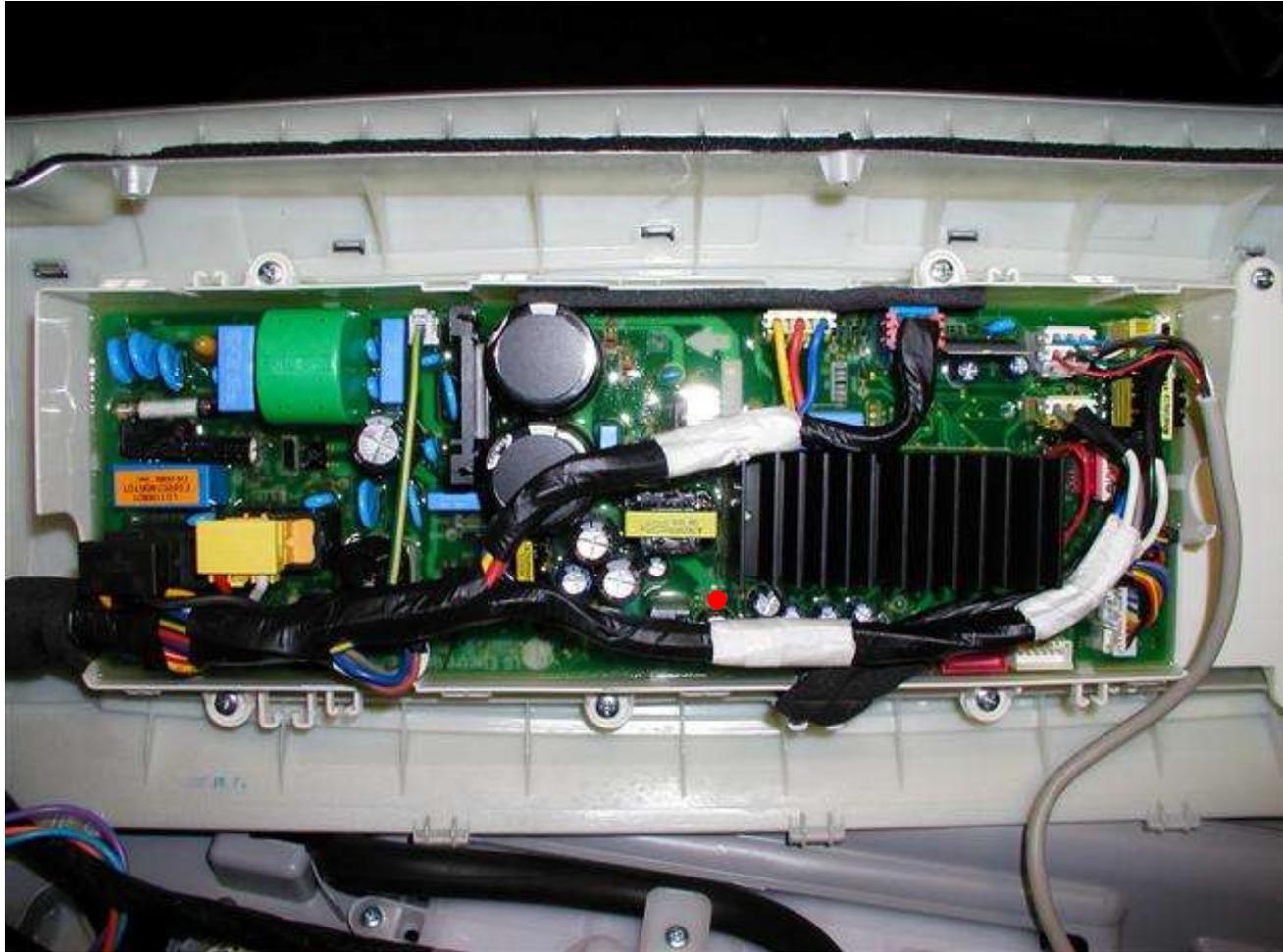
Removing the metal cover will expose the plug connections and the individual electronic components on the power board.
