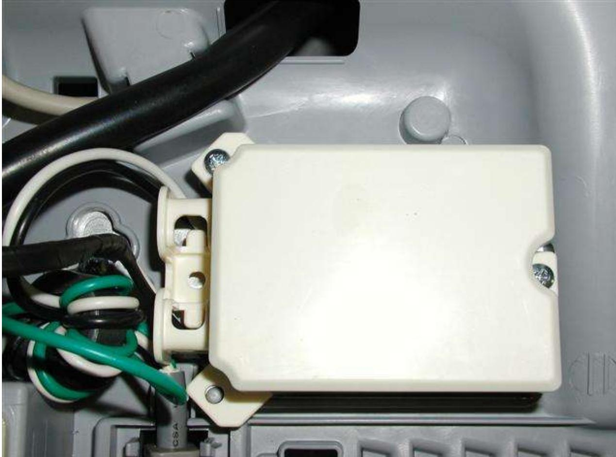
Noise filter helps to block out line noise that could adversely affect the washer control system.
