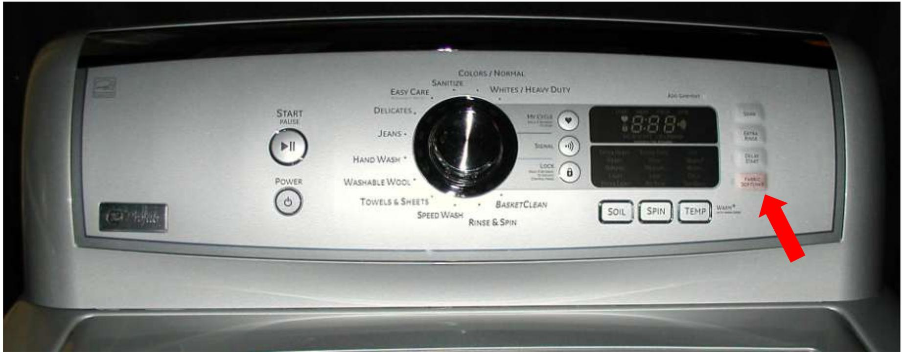
When the fabric softener pad is selected, the machine will provide a deep rinse instead of the spray rinse.
