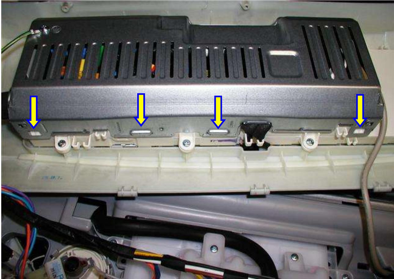
To remove metal shield from control board assembly, pull outward on side tabs.
