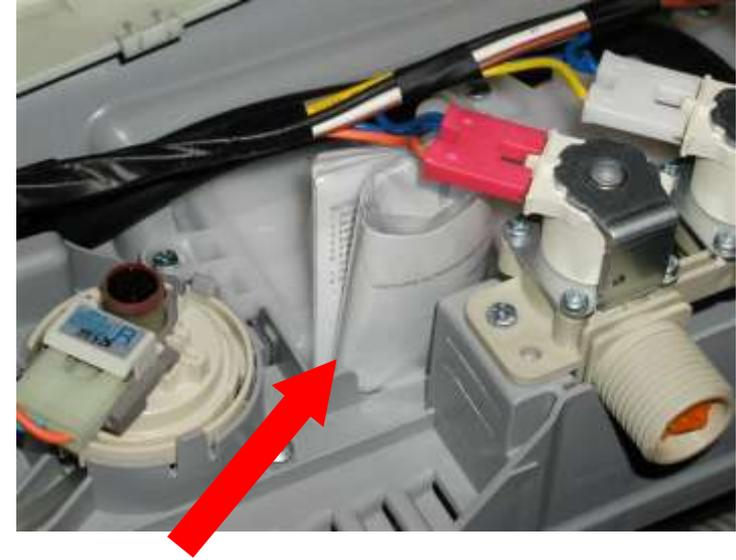
Mini-Manual is packaged inside a plastic bag and is located inside the backsplash between the pressure switch and the water valve assembly.
