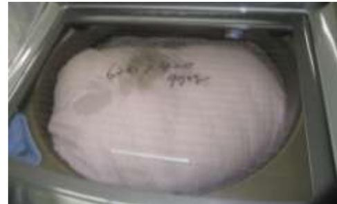
Worst case scenario in testing was with an overloaded tub with a pillow or pillows at the top of the load.
