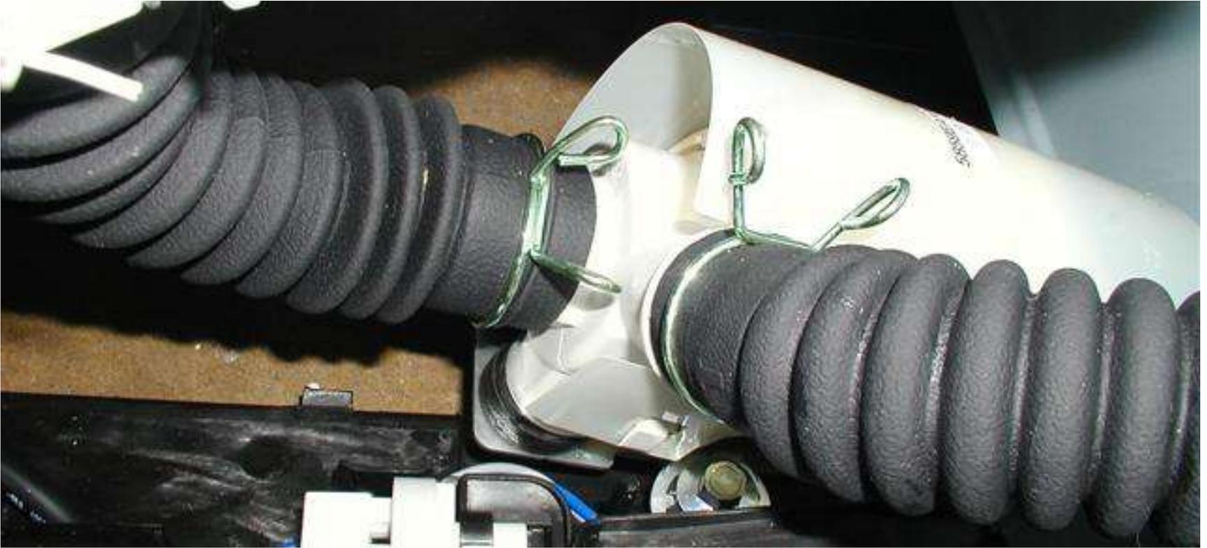
**Note:** The drain hoses are difficult to remove due to a sealing compound used at the factory.
