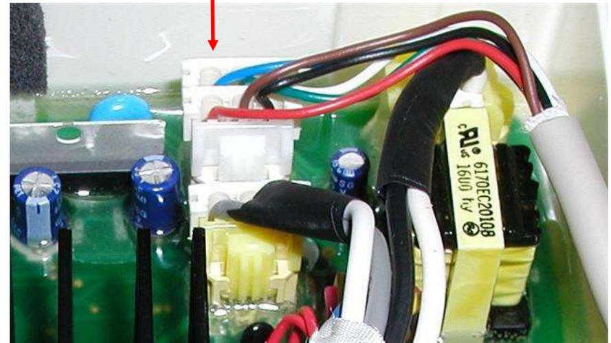
Lid lock assembly is secured to the underside of the washer top with two Phillips screws. The assembly includes the interconnect cable and plug. It connects to a six pin connector on the Main PCB at the plug shown above.
