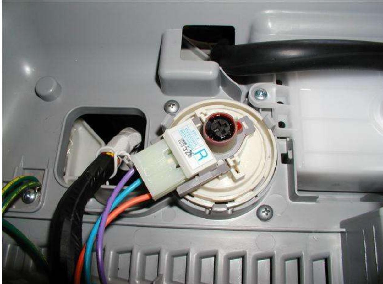
The pressure sensor is connected by a clear hose to an air reservoir near the bottom of the outer tub and operates by a frequency (kHz) signal to the main control board.
