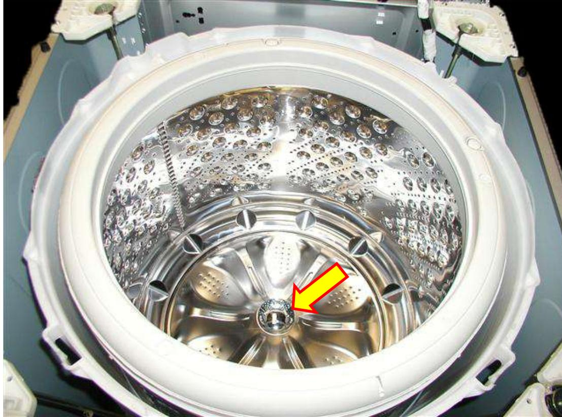
Place a flat blade screwdriver in the slot under the infusor cap and gently pry off.
