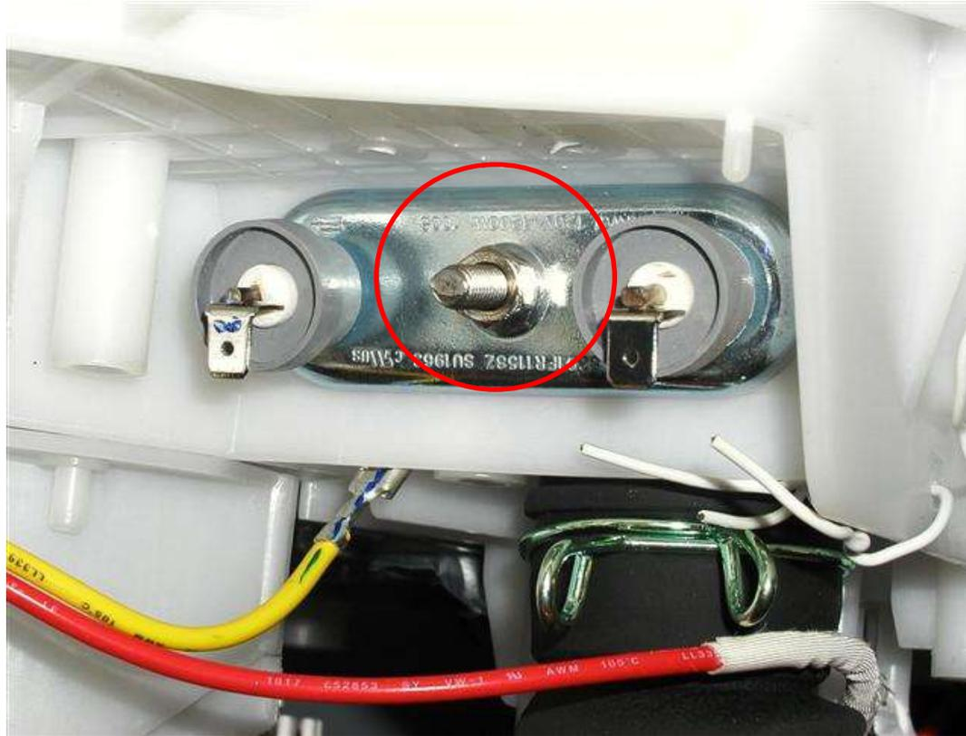
**CAUTION:** Proper torque must be applied to the 10mm hex nut in order to assure a proper seal. Under torque could cause water leakage, over torque could cause the tub to crack.
