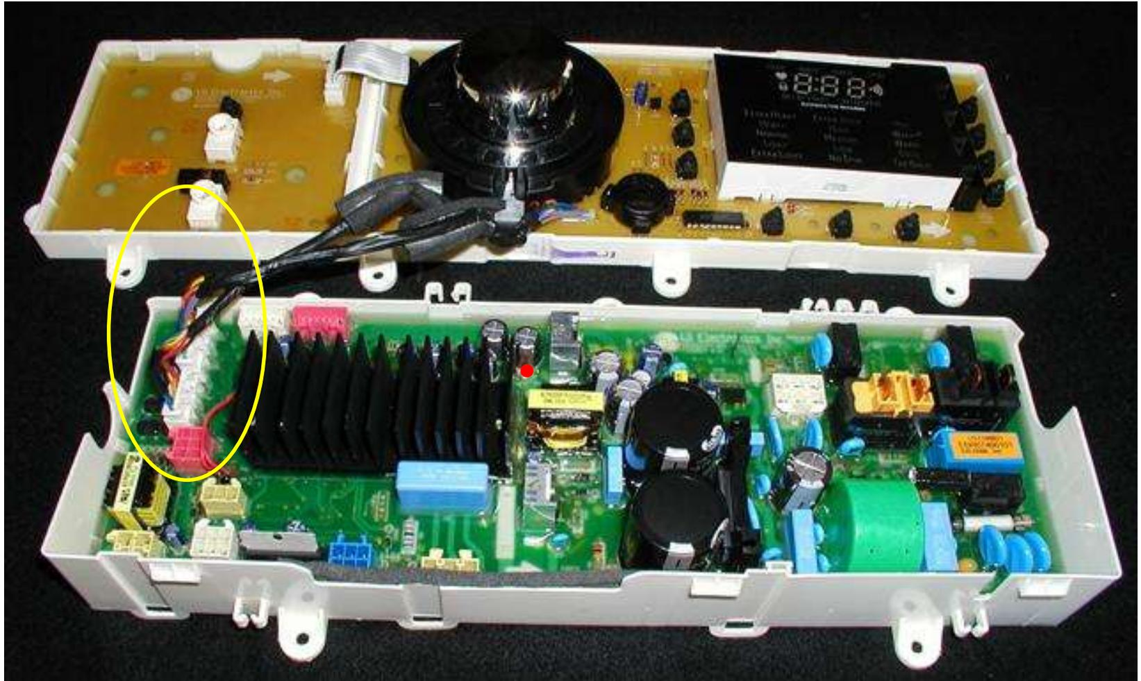
Finally, disconnect the two electrical connectors from the Power Board.
