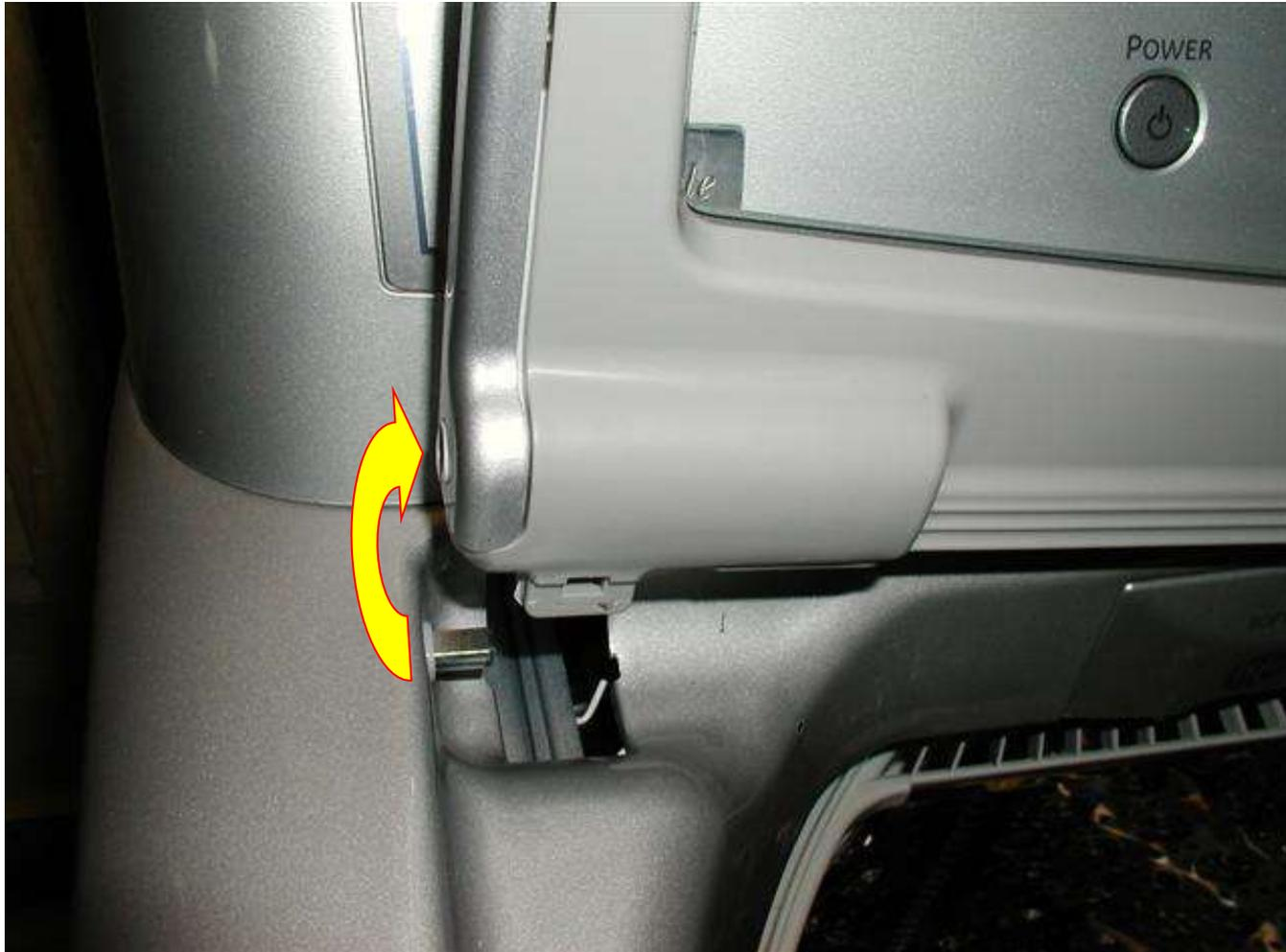
With hinge pin pulled completely to the left, lift left side of the lid upwards to clear pin....
