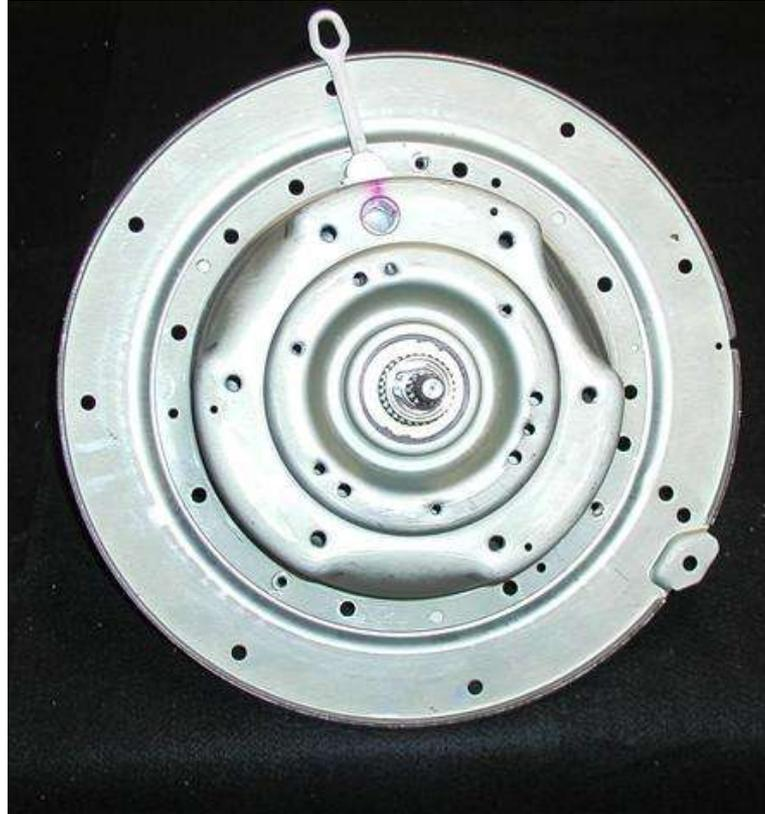
Remove the bearing housing assembly.
