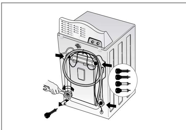
2. Unscrew the 4 bolts with the wrench supplied.
