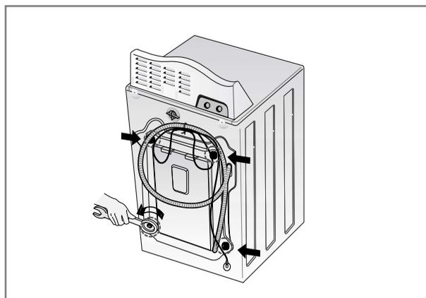
3. Take out the 4 bolts and braces by twisting the braces slightly. Keep the 4 bolts, braces and the wrench for future use.
