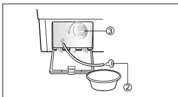
3. Remove out any foreign objects from the pump filter (③). After cleaning, turn the pump filter (③) clockwise and insert the drain plug (②) to the original place. Close the lower cover cap (①).
