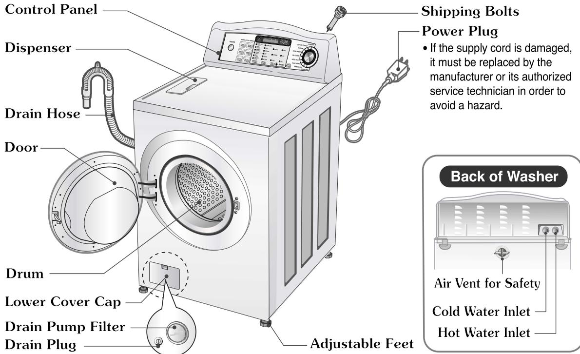
• If the supply cord is damaged, it must be replaced by the manufacturer or its authorized service technician in order to avoid a hazard.
