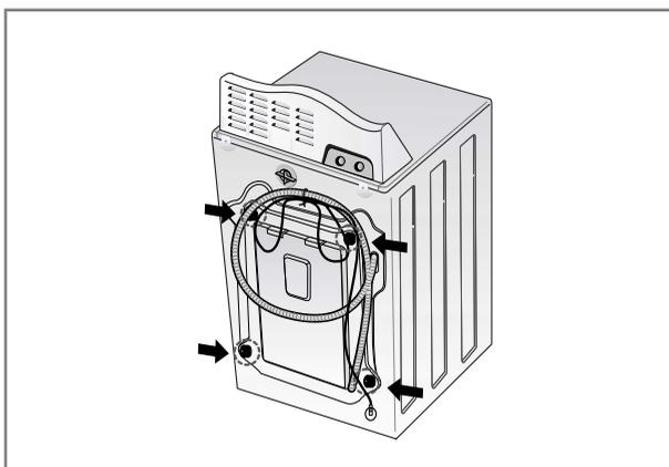
1. To prevent internal damage during transport, the special 4 bolts are locked. Before operating the washer, remove the bolts and braces.
