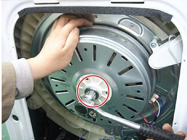
Slide a Philips screw driver into a hole in the rotor and through a stator winding. This will keep the rotor from spinning the drum when loosening the nut. Using a 19mm wrench or socket, remove the retaining nut and washer
