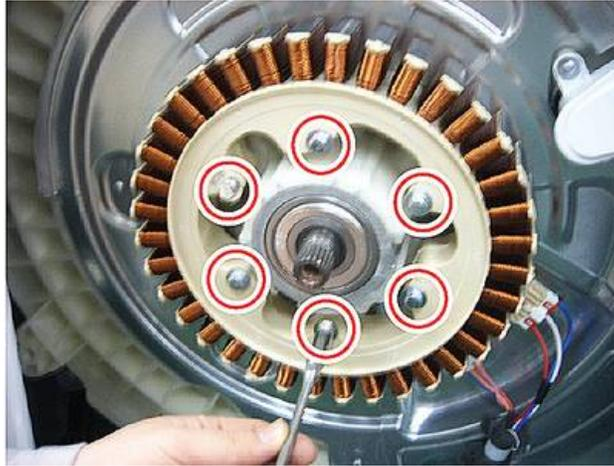
Remove the 6 - 10mm bolts that secure the stator to the rear tub section
