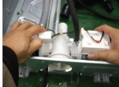
Disconnect the wiring harness connectors to the drain and circulation pump sections and remove both as an assembly. Install the new pump following the reverse order of this procedure.
