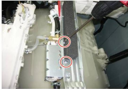
Remove the screws that secure the steam unit to the frame of the machine
