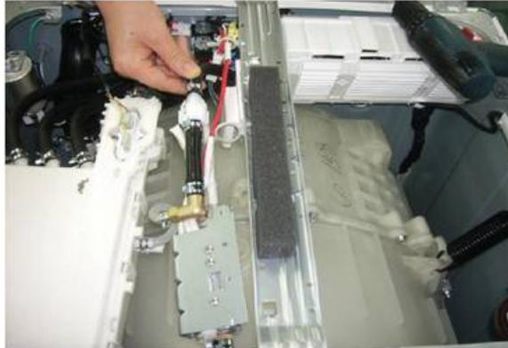
With the screws removed, disconnect the wiring harness and water lines to the steam unit and remove. Reverse the procedure to install the new steam unit.
