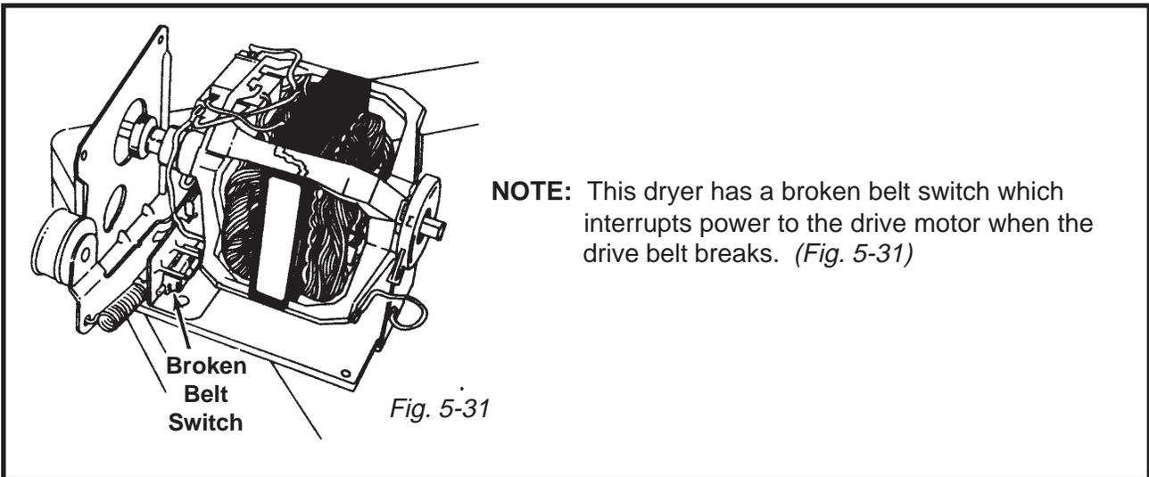
**NOTE:** This dryer has a broken belt switch which interrupts power to the drive motor when the drive belt breaks. (Fig. 5-31)
