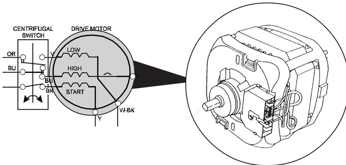
Check the high-speed windings by testing between the blue and white wires. A resistance reading between 3/4 ohm and 2 ohms should be present.
