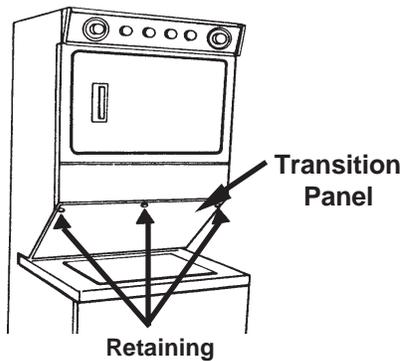
2. Release the two washer top retaining clips and slide the washer top forward off the unit. (Fig. 5-16)
