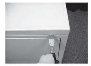
3. Disconnect wiring from the Door Switch.
