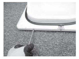
5. After Door Panel screws are removed the Door Gasket can be removed from the Inner Door Panel.
