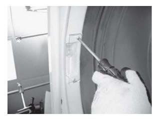
4. Depress locking tab on Light Socket and remove through light cavity.
