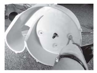
13. Remove Motor locking collar front and back to remove Motor.
