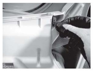
5. Remove three screws inside drum retaining Blower Duct.
