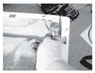
6. Tip Front Panel back and remove. Rotate Front Panel to the back side and remove gasket.
