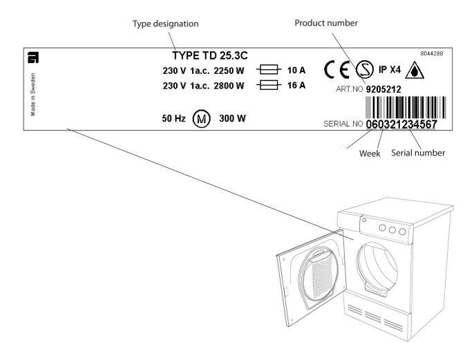
It should be easy to service a tumble dryer. It is important that you, as a service technician, are given the conditions to be able to carry out work in an efficient and satisfactory way. Our hope is that this service manual is a useful tool for your daily work.
