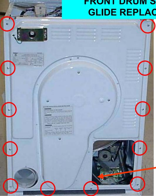
To replace the front drum support glides, remove all screws holding the back panel in place
