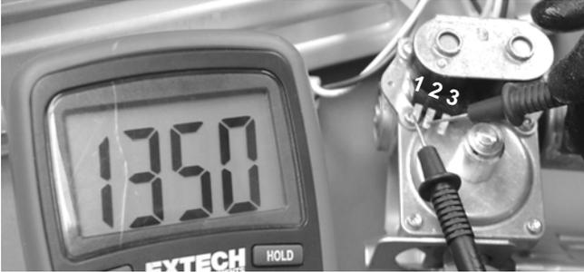
Check the holding coil across terminals #1 and #2. Resistance should be approximately 1350 OHMS
