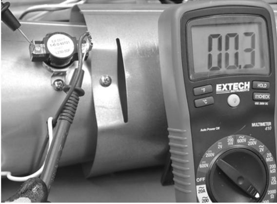
TH2 is a normally closed Hi-Limit safety. The resistance across the terminals should be less than 1 OHM
