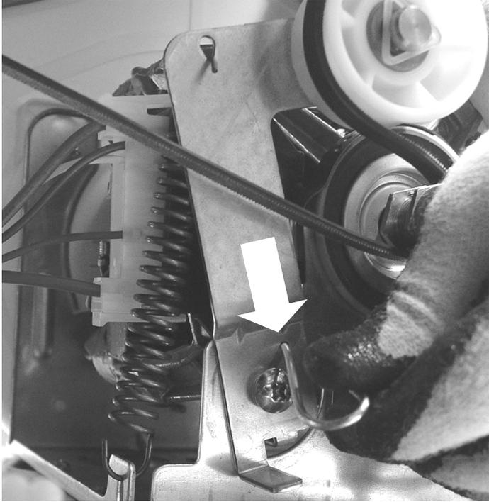
On completion of the reassembly, remove the locking rod
