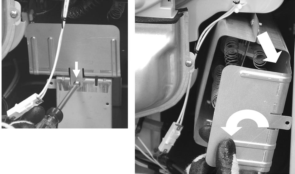
Remove screw, rotate heater assembly and pull out
