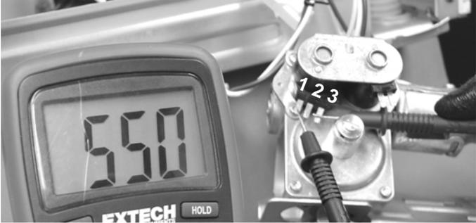
Check the booster coil across terminals #1 and #3. Resistance should be approximately 550 OHMS
