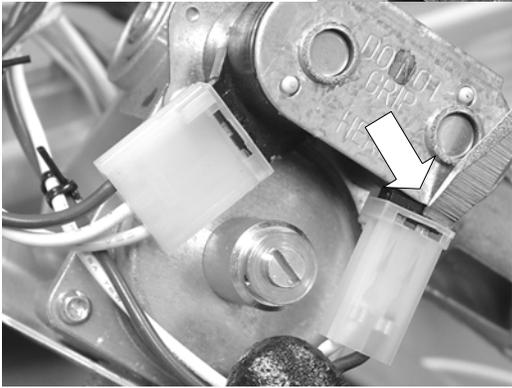
Use a screwdriver to release wire connectors from valves
