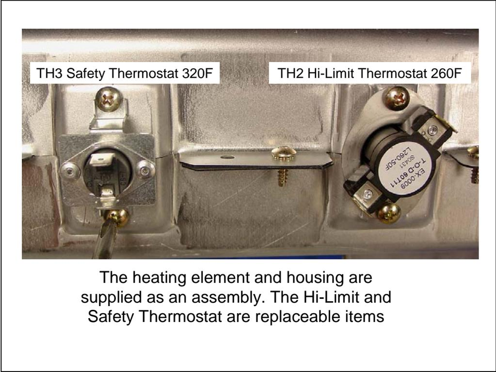
**Slide 46 - Installing the Heater Assembly**
