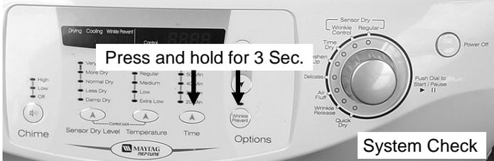
The image shows the control panel of a Maytag dryer. A white box with the text "Press and hold for 3 Sec." is overlaid on the Time and Wrinkle Prevent buttons. A label "System Check" is in the bottom right corner of the panel image.
