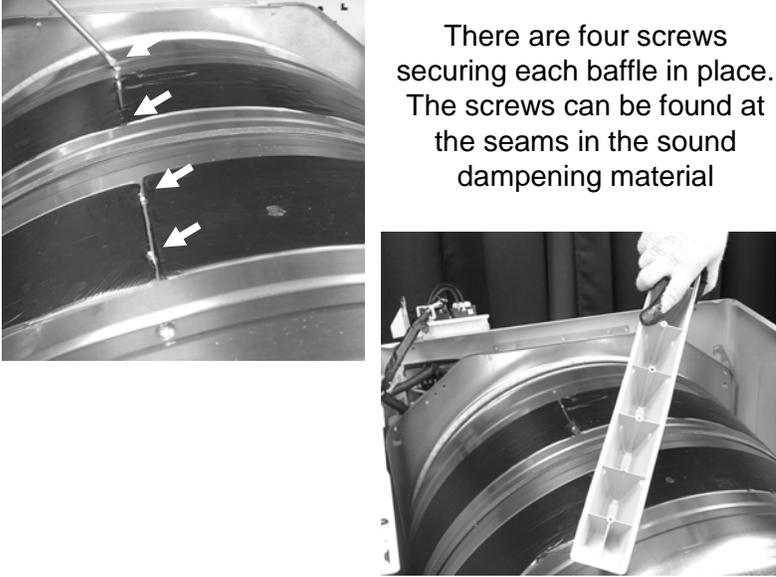
There are four screws securing each baffle in place. The screws can be found at the seams in the sound dampening material
