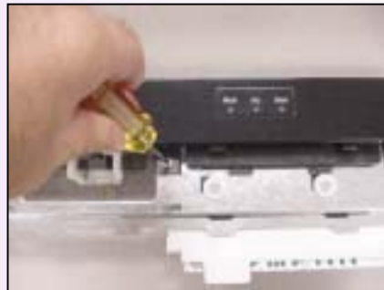
Removing fascia screws
