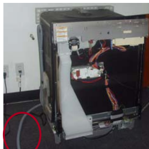
Lie drain hose on the floor → Hose position is below than 10"(250mm)
