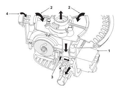
5. The main wash pump then stops, creating positive pressure in the pump's inlet chamber. This opens the check valve allowing the remaining water to be drained away. **(5)**
