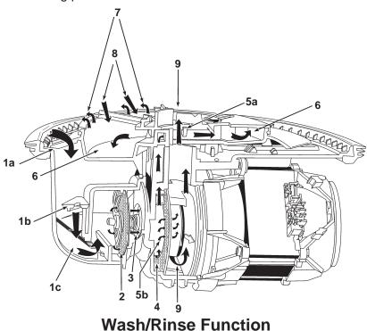
The main wash water passes from the spray arm nozzles, over the dish load and into the sump assembly, where a number of operations occur.
