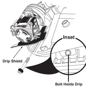
Fig. 3-20 Shield in Place
