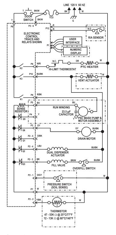
**NOTE:** Check Strip Circuits for resistance and wattage values.
