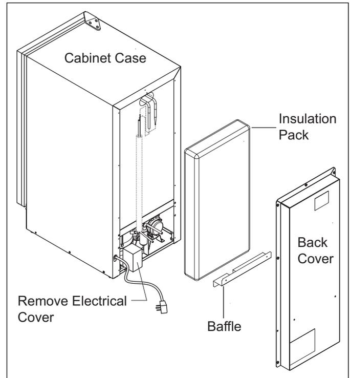
**Figure 5-6 Power Cord Removal**
