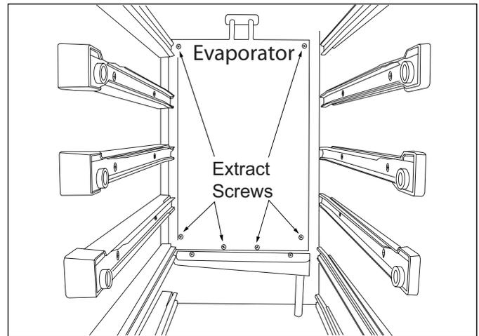
**Figure 5-14. Evaporator Removal**
