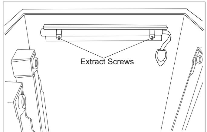
Figure 5-11 . Light Bulb and Housing Removal
