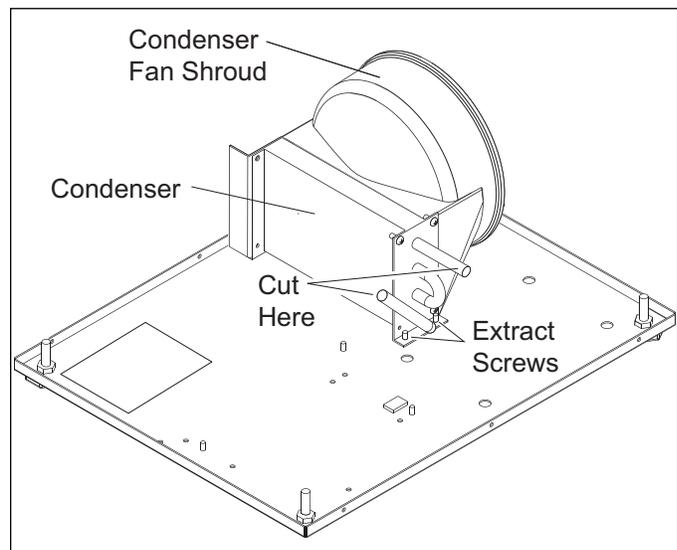
**Figure 5-17. Condenser Removal**
