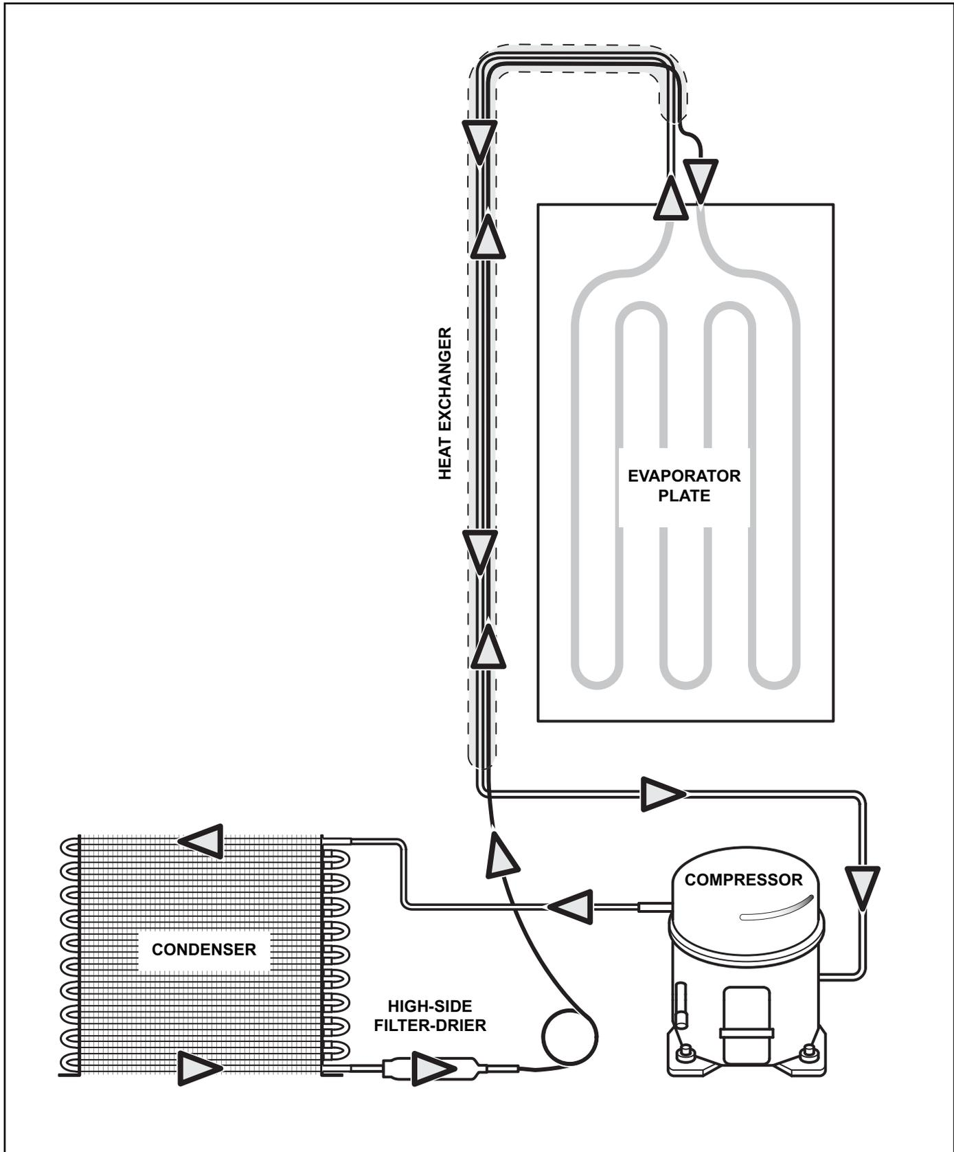
Figure 4-7. Model 315W Refrigerant Flow
