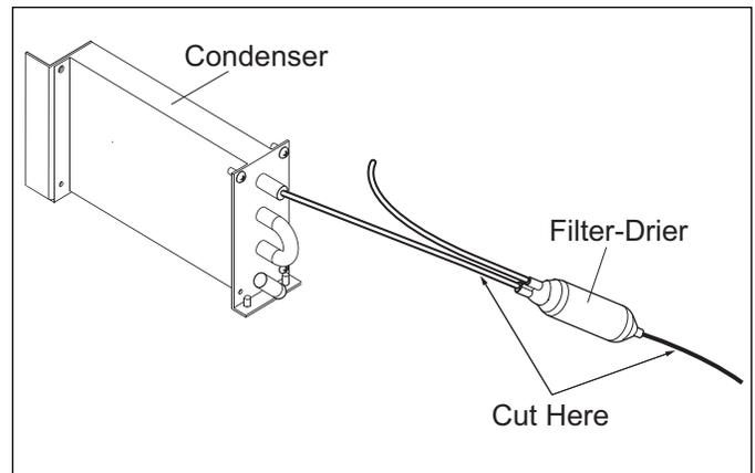
**Figure 5-15. Cut Drier Inlet & Outlet**
