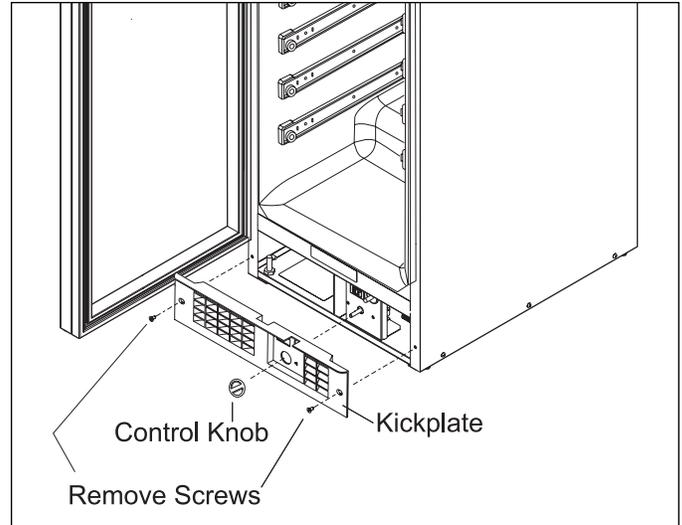
Figure 5-1. Kickplate Removal
