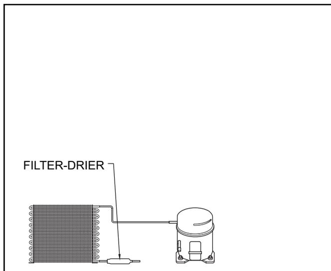
Figure 4-3. Filter- Drier
