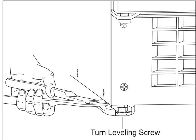
**Figure 2-5. Unit Leveling**
