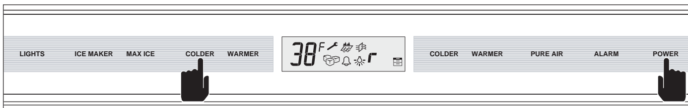
Figure 3-80. Initiate Diagnostic Mode First - Press and Hold Either COLDER Key, Then the POWER Key
