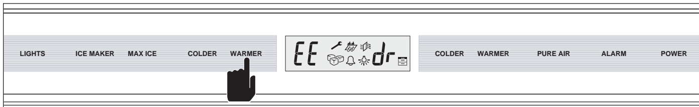
Figure 3-65. Currently no Thermistor in Drawer Area, so “EE” will Appear to the Left of the “dr”
