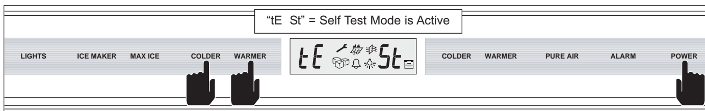
Figure 8-2. Initiate Self-Test Mode - While in Diagnostic Mode, Press COLDER, WARMER and POWER Keys
