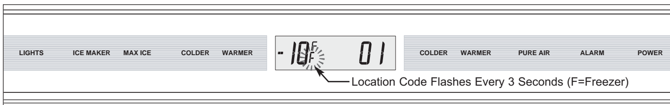
Figure 3-72. Thermistor Location Code Flashes at 3 second intervals (F then E = Freezer Evaporator)
