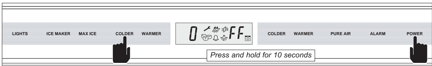
Figure 3-88. Initiate Manual Component Activation Mode for Freezer Components - While in Diagnostic Mode, Press and Hold Freezer COLDER and POWER for ten (10) seconds, Then Press Freezer WARMER or COLDER Key to Activate Components as Indicated in Table
