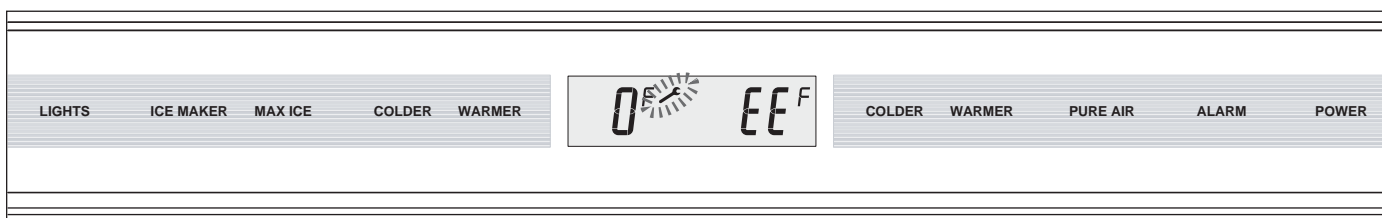
Figure 3-55. Service Icon Flashing and "EE" at Right = Refrig. Compartment Thermistor (or its wiring) Fault
