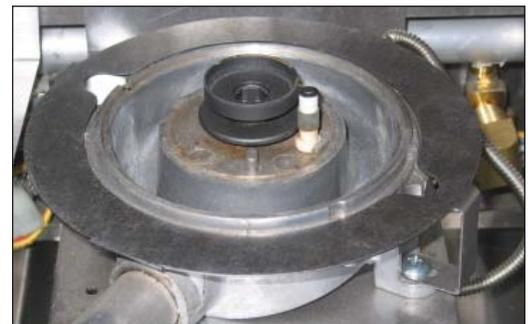
Picture 3 Diverter Installed
