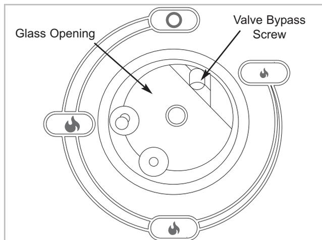
**Figure 2A. Valve Bypass Screw (International)**
