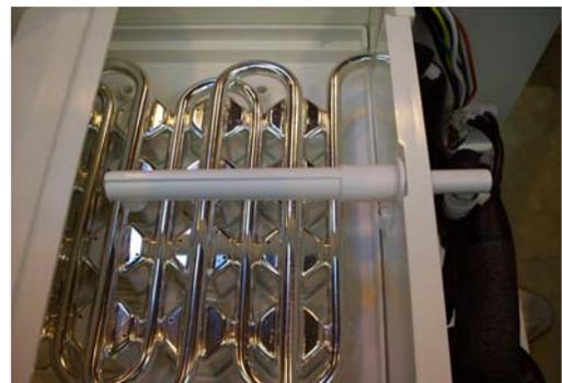
During the last minute of the freeze cycle the control board took another set of temperature readings and calculated how long it should take to harvest 16 cubes of ice.
