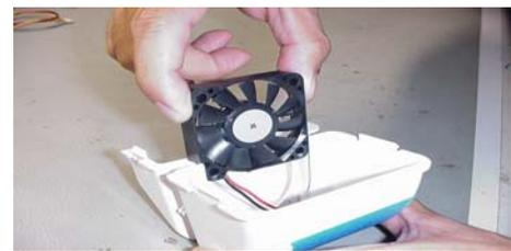
Handle impeller from sides for inspection
