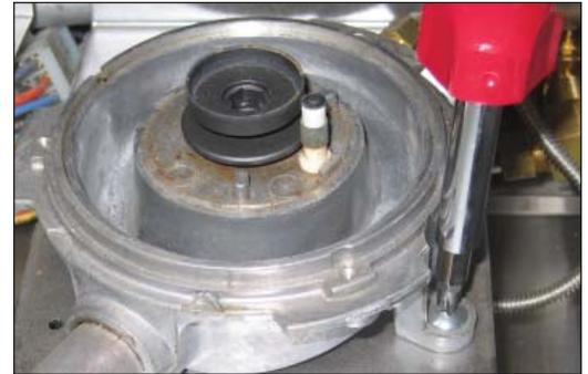
Picture 1 Burner Screws
