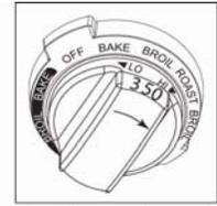
Turn Knob to Right for Preset Temperature or to Select Desired Temperature
