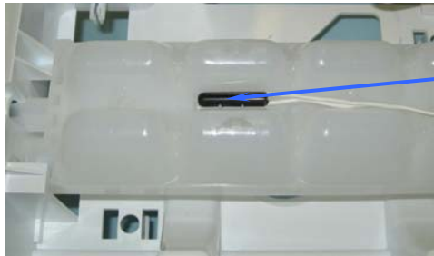
Icemaker sensor located under insulated pad.
