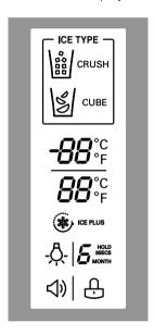
\* LED check function : If simultaneously pressing Ice Plus button and freezing temperature adjustment button for a second, display LED graphics on. If releasing the button, the LED graphic displays the previous status.
