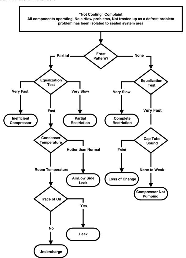
(The equalization test is trying to restart a compressor using a start kit after it has been operating.)
