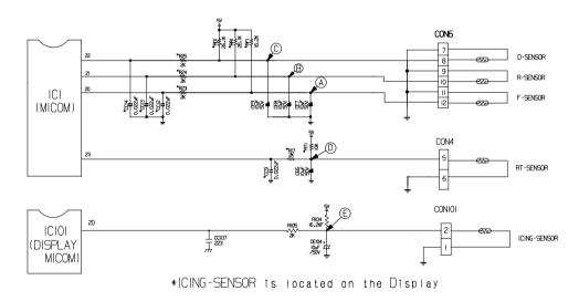
The upper circuit reads refrigerator temperature, freezer temperature, Icing sensor temperature and defrost sensor temperature for defrosting and the indoor temperature for compensating for the surrounding temperature into MICOM. Opening or short state of each temperature sensor are as follows:
