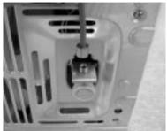
2) Separate the Mechanical Cover and Valve Screw.
