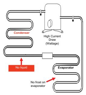
Low side leak, air in system
