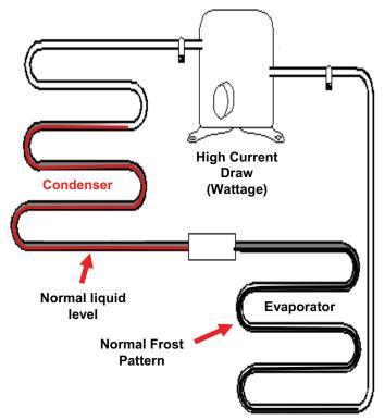
Conditions that mimic a sealed system failure:
