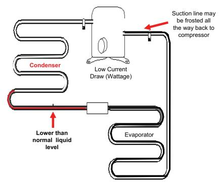
Conditions that mimic a sealed system failure:
