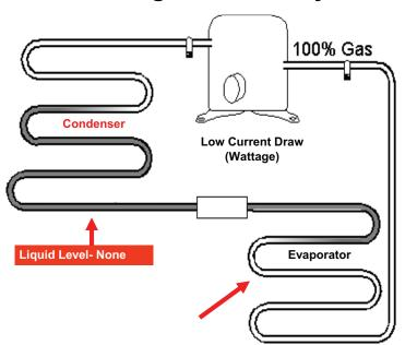
High Side Leak- No refrigerant left in system.
