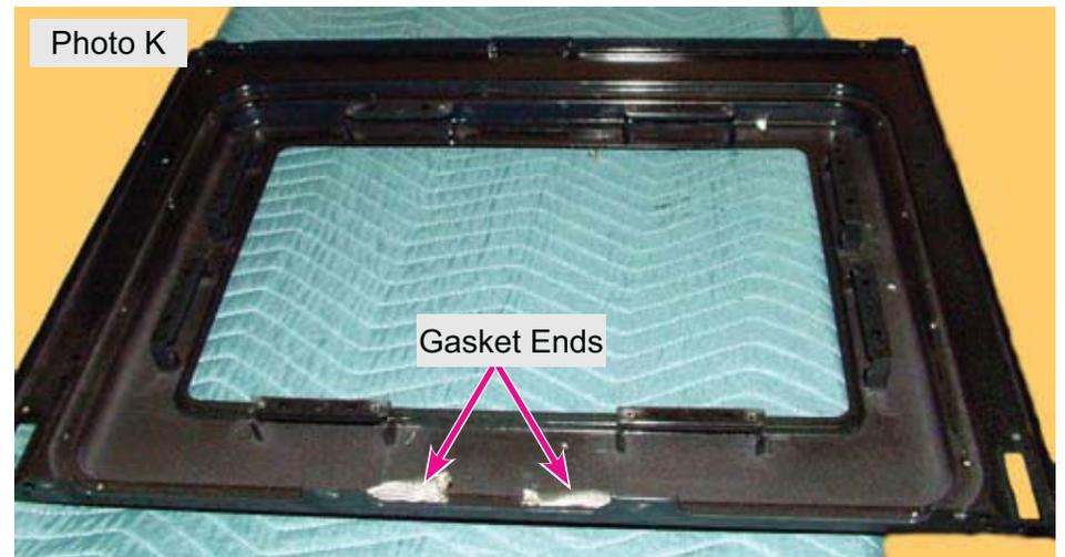
The gasket is secured to the liner by metal spring clips that can be pulled out from the opposite side (photo L).
