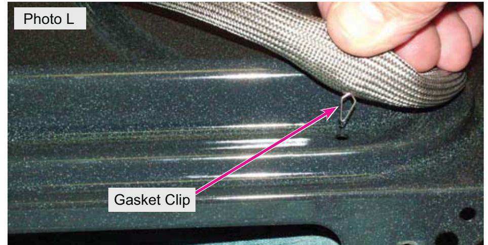
Note: Be sure to re-insert the loose ends of the gasket into the holes at the bottom of the door liner before reinstalling the inner door glass panes or insulation (photo M).
