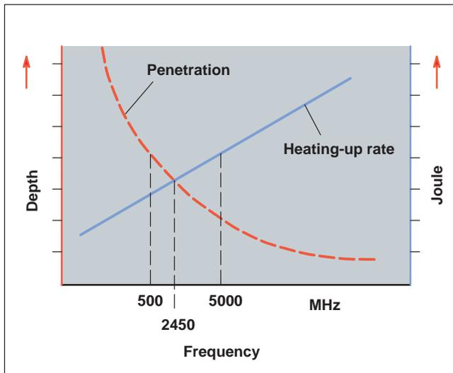
Fig. 13 Penetration depth and temperature gain as a function of frequency
