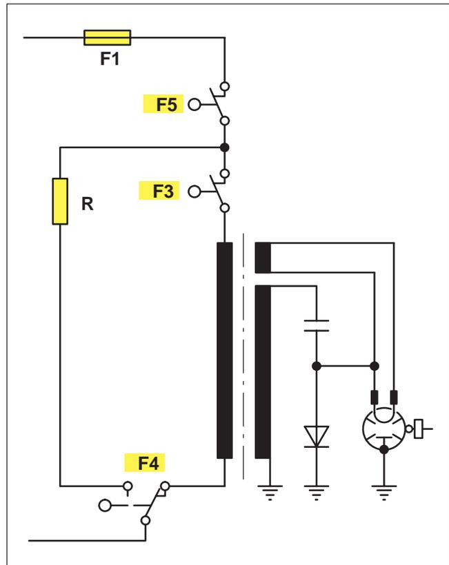
Fig. 63 Safety circuit (door closed)
