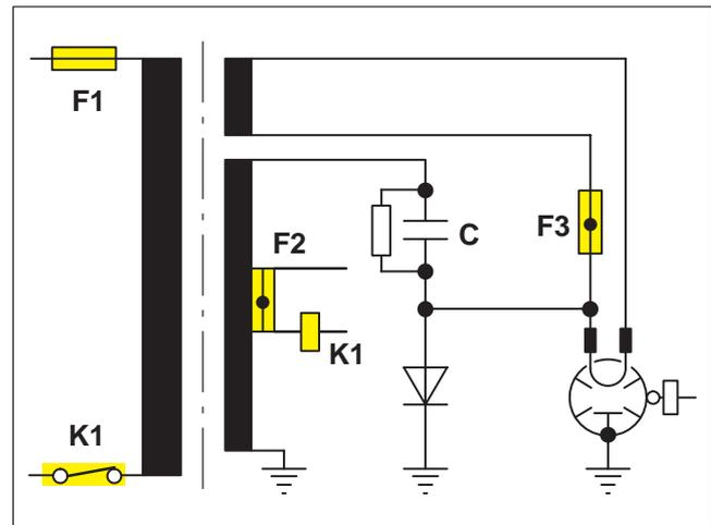
**Fig. 45 Protective circuit by means of transformer fuses and wire fuses**
