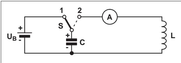
Fig. 24 Anti-resonant circuit
