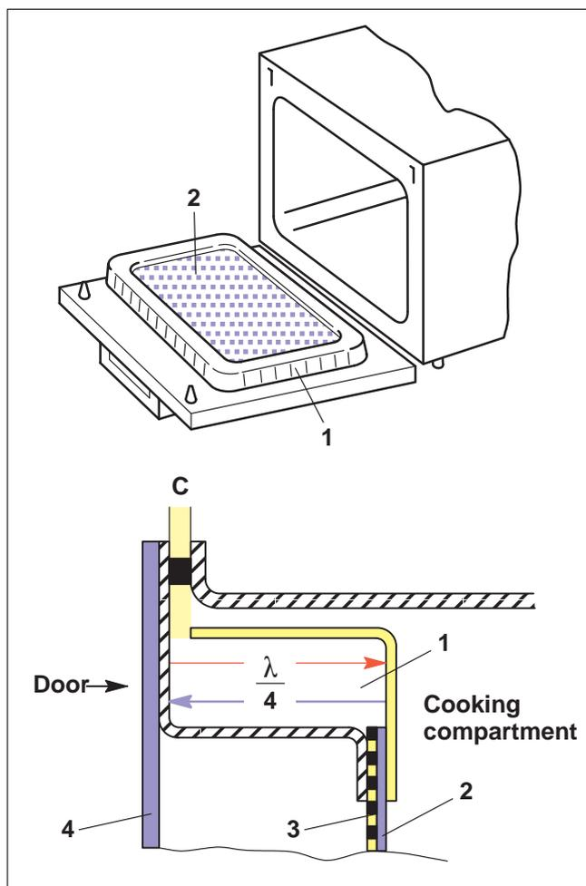
**Fig. 70** Sealing system with an internal, horizontal lambda trap
