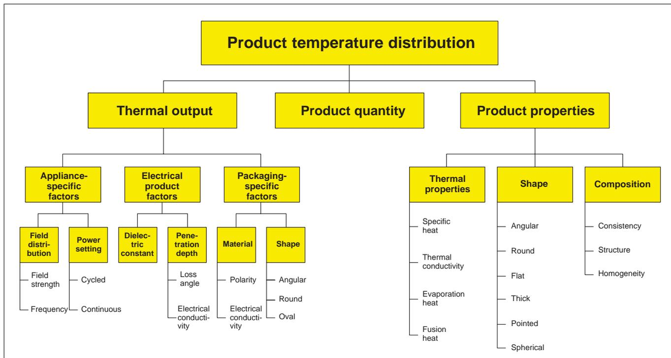
**Fig. 23 Factors which influence the temperature distribution in products**
