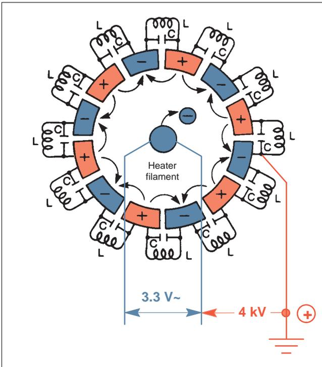
**Fig. 37 Oscillating circuit**
