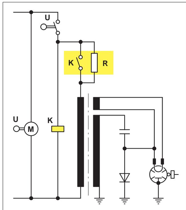
Fig. 59 Inrush current limiter for appliances with electromechanical control
