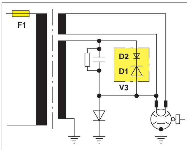
**Fig. 47 Protective diode**
