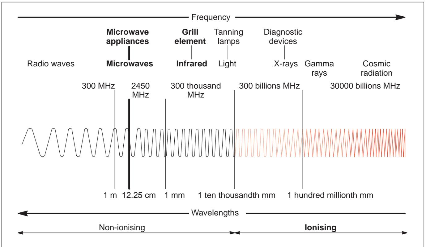
**Fig. 7 Application areas for electromagnetic waves**
