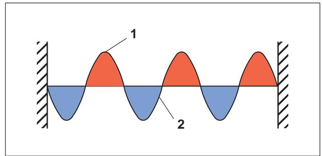
**Fig. 73 A standing microwave in the cooking compartment**
