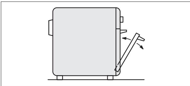
**Fig. 78 Door operation 100,000 times**
