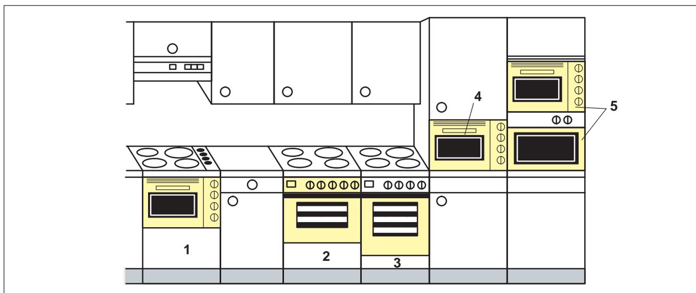
**Fig. 88** Installation options for microwave appliances
