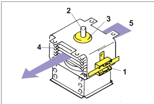
**Fig. 65 Magnetron with temperature limiter**
