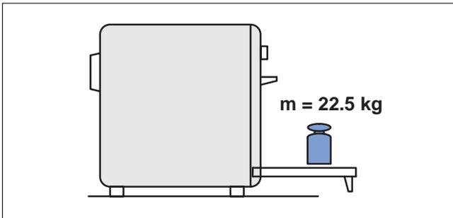
**Fig. 79 Mechanical loading of the door**
