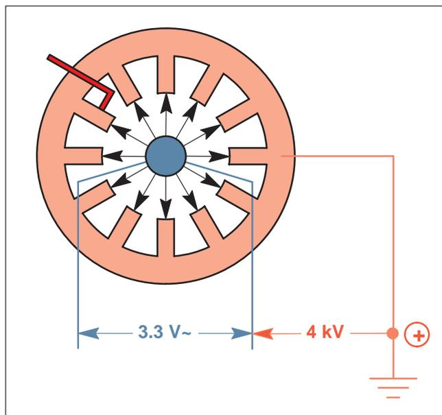
**Fig. 34 Flow of electrons**
