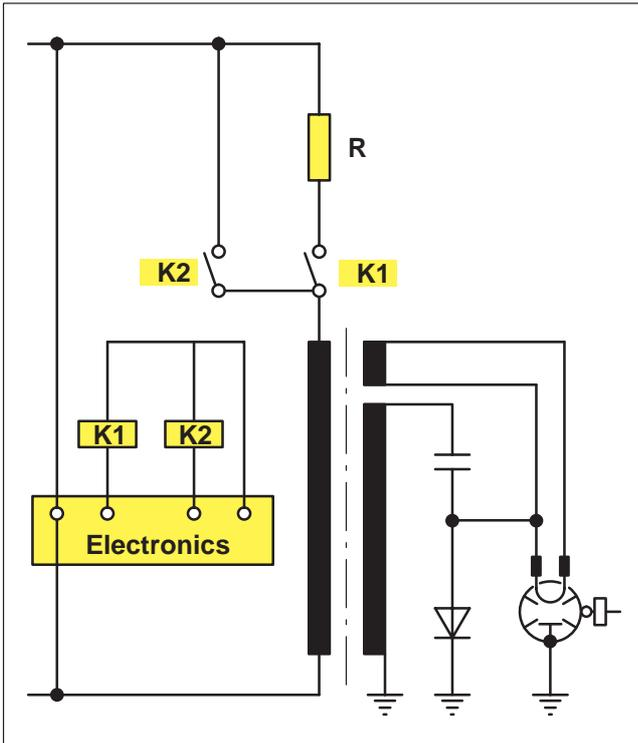
**Fig. 60 Inrush current limiter for appliances with electronic control**
