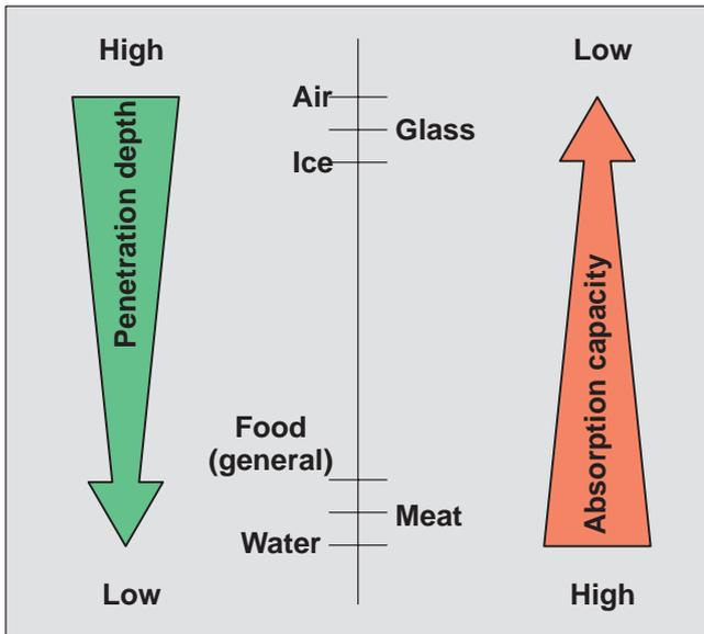
**Fig. 15 Penetration depth and absorption**
