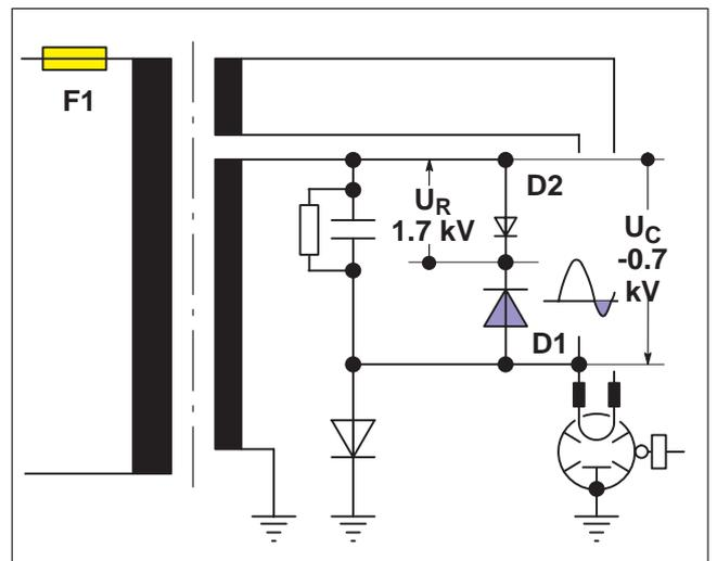
**Fig. 49 Normal situation: capacitor voltage  $U_C = -0.7$  kV**
