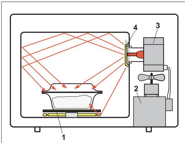
**Fig. 75 Microwave distribution with rotary base**
