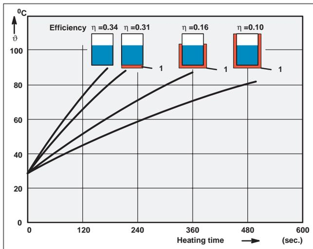
**Fig. 9 Influence of metal screening on heating, time and efficiency**
