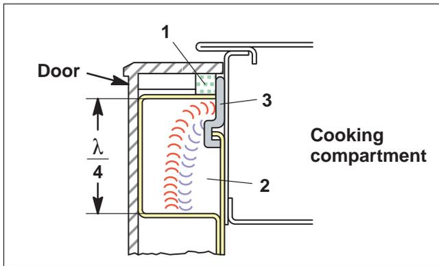
**Fig. 72 Ferrite seal and external Lambda trap**
