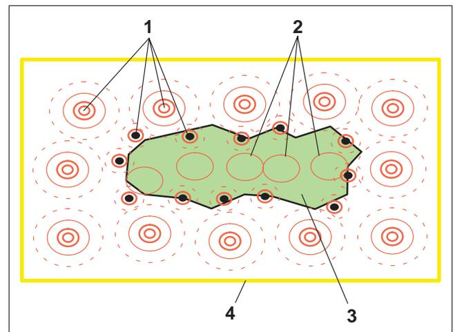
**Fig. 22 Energy distribution on a cooking compartment plane, with food**
