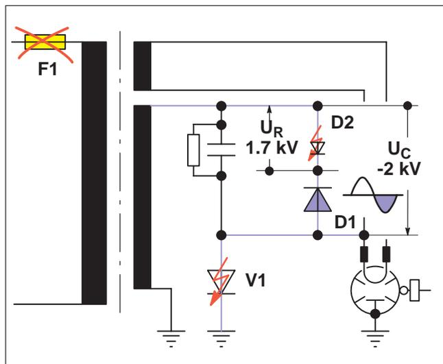
**Fig. 50 Fault situation: short-circuit in high voltage circuit**
