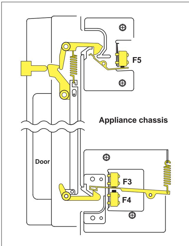
Fig. 62 Door safety switch arrangement for a microwave appliance (door closed)
