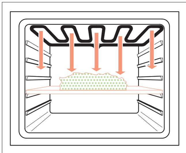
**Fig. 5 Thermal radiation from a grill element**
