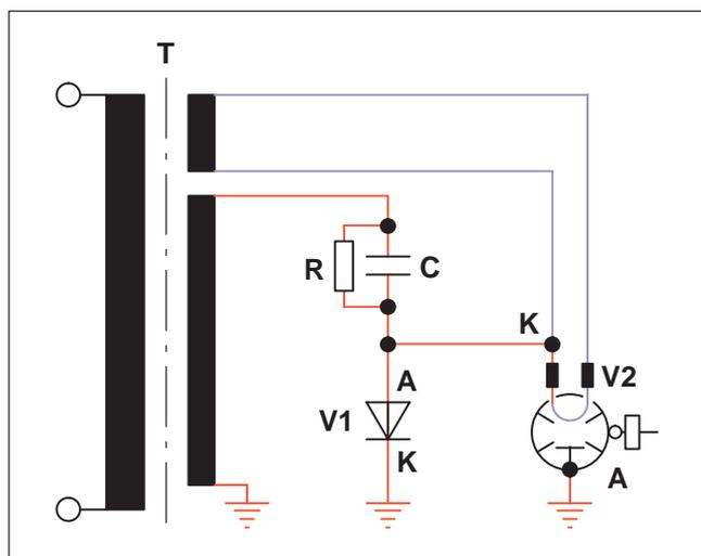
Fig. 39 Voltage doubler circuit
