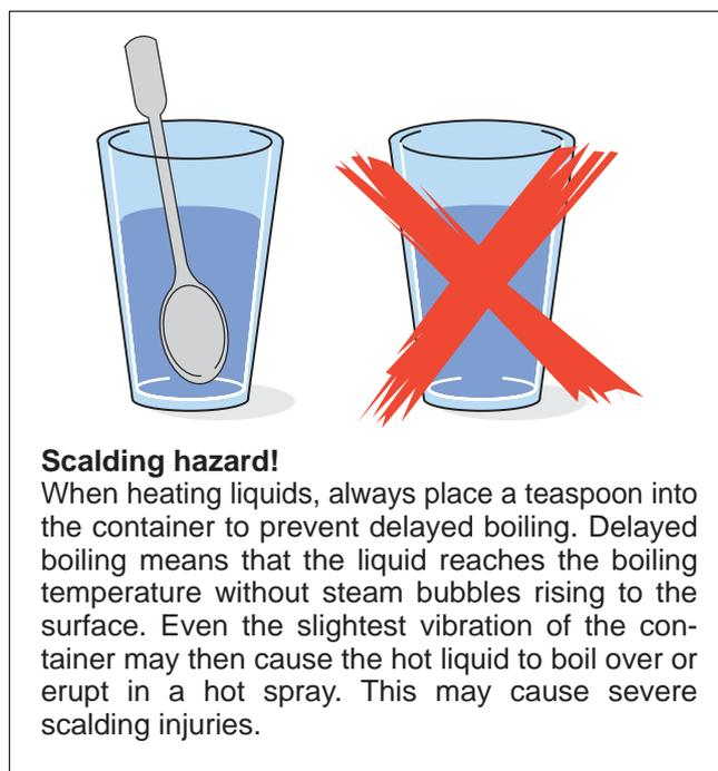
**Fig. 90** How to prevent delayed boiling
