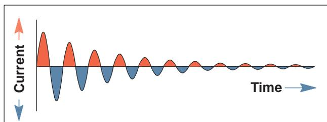
**Fig. 26 Damped oscillation**
