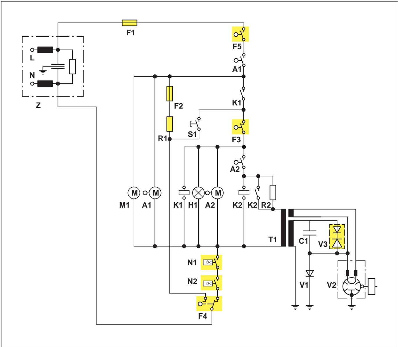
Fig. 66 Main wiring diagram for a microwave appliance with electromechanical control
