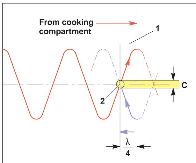
**Fig. 71** Lambda trap functional principle
