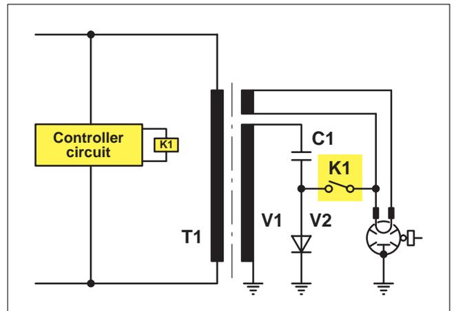
**Fig. 56 Cycling on the secondary side**
