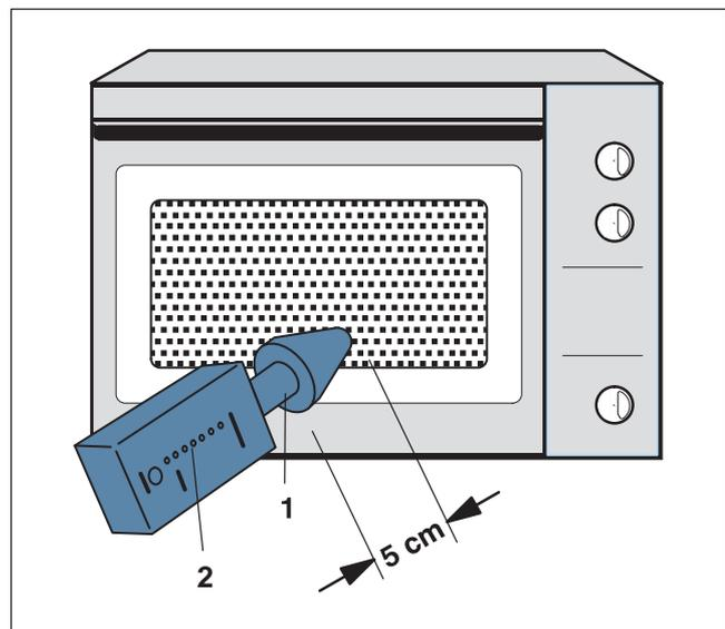
Fig. 84 Example of a sealing test
