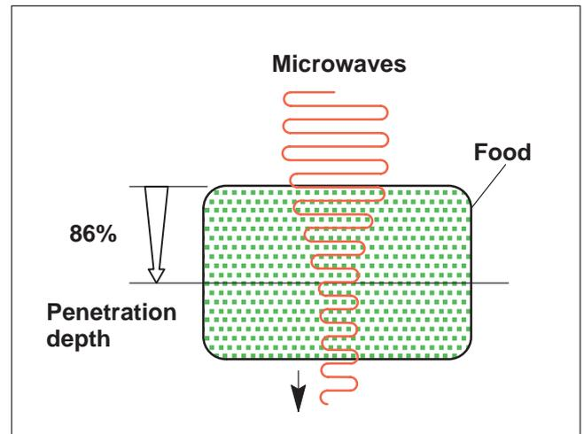
Fig. 14 Penetration depth
