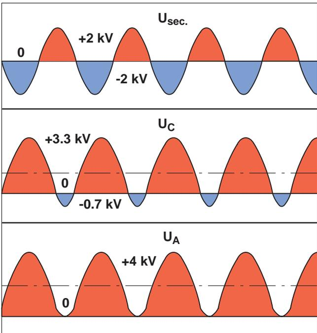
Fig. 42 Voltage waveshape during microwave operation
