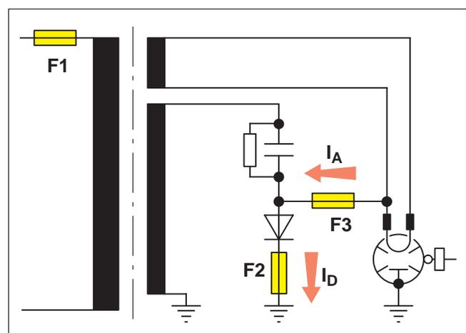
**Fig. 46 Fuses in the diode and anode current circuits**
