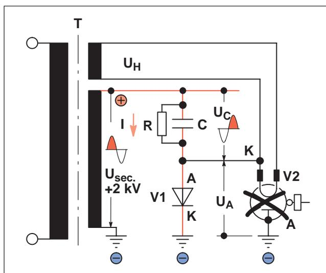
Fig. 40 Doubler circuit during 1st positive half-wave
