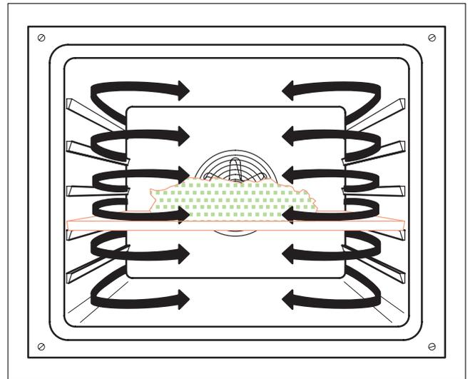
Fig. 3 Heat flow by means of forced convection for a fan-assisted oven
