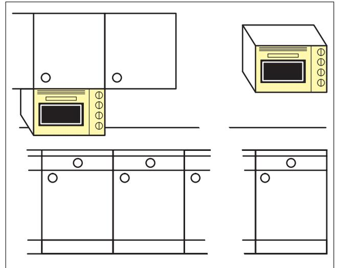
**Fig. 86 Top cabinet and wall mounting**
