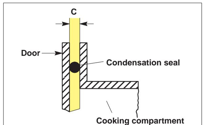
Fig. 69 Capacitive seal
