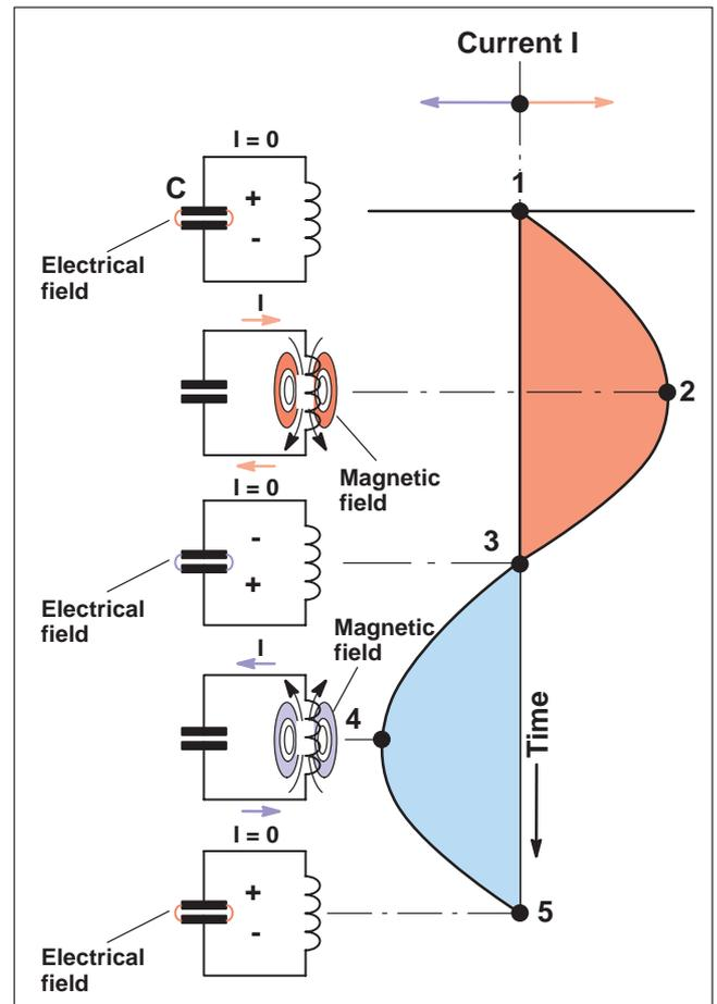
Fig. 25 Progress of an oscillation
