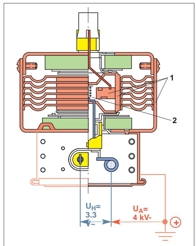
**Fig 33 Magnetron voltage supply**
