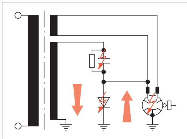
**Fig. 44 Short-circuit on the secondary side**
