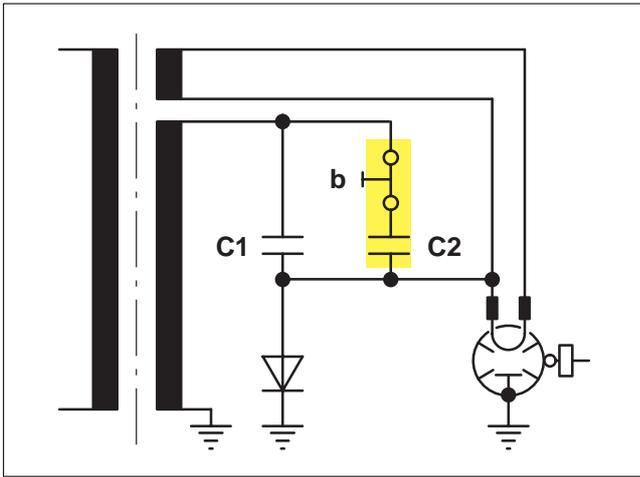
**Fig. 53 Power control by changing the capacity of the high-voltage capacitor**
