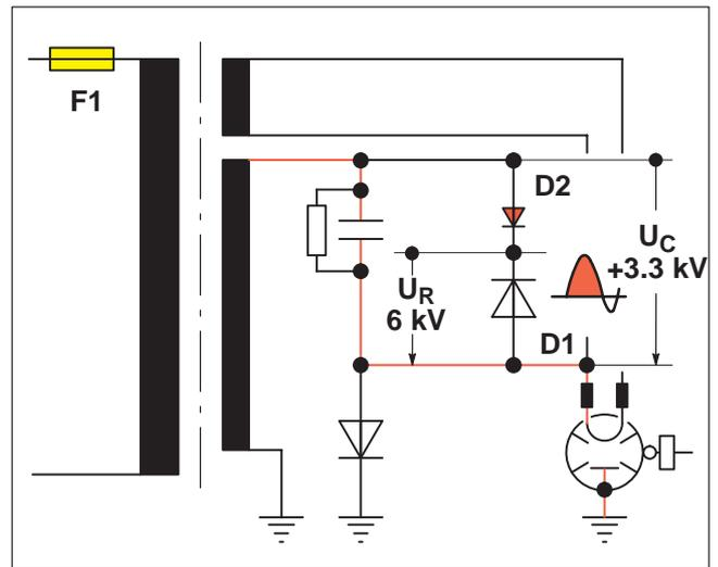
**Fig. 48 Normal situation:  $U_C = +3.3$  kV**
