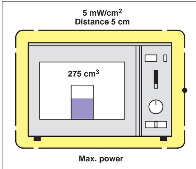
Fig. 82 Normal operation with load
