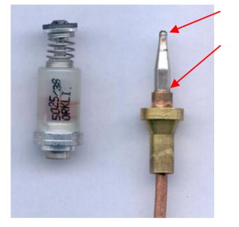
There are many types of thermocouples and magnetic valves in existence. These are differentiated by, among other things, electrical, thermo-electrical and mechanical properties (retaining current, level and run-up behaviour of the thermo-electromotive force, retention or throw-off force of the solenoid valve). Within appliances, these versions are combined and checked along with the existing burners to ensure that the required system function is provided.
