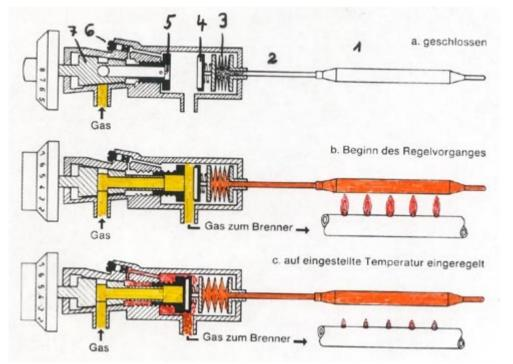
In cold state, the flow of gas through this valve disk is maximised, irrespective of the temperature setting. The maximum burner output channelled through is determined by a main nozzle located externally (in the oven burner). As the sensor heats up, the valve disk is pushed back by the bellows and the volume of the gas flow is gradually reduced.
