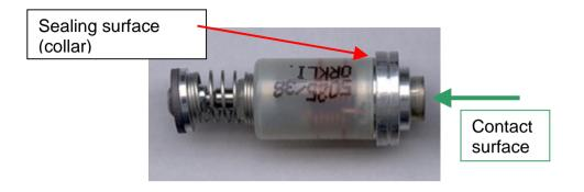
The valve disk, pull-back spring, armature plate and magnetic coil are integrated in the magnetic insert. In the case of gas taps with a thermal release, this magnetic insert can be replaced as a spare part.
