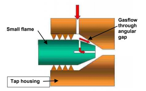
Condition: the bore of the existing nozzle at the fixed end stop must give rise to a smaller gas flow than is required for the burner.
