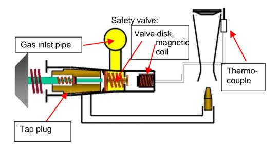
In the off position, the safety valve disk is pressed against the endstop by the spring, thus closing off the flow of gas into the tap. Accordingly, in the off position there is no gas pressure at the tap plug. Any leak in the area of the tap plug would therefore have no effect:
