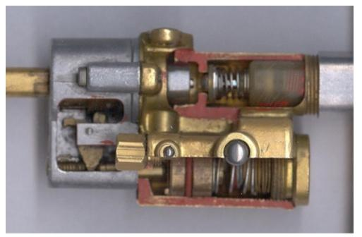
The set turning angle for the operating spindle (temperature preselection) tensions a counterpart against the valve disk by means of a spindle and push-rod system, thus influencing the volume of gas flow and, in the final analysis, the prevailing temperature in the oven.
