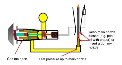
If, with the nozzle sealed off (blocked with a finger or pencil, main nozzle fitted with solder seal), the actuator is opened, a slight fall in pressure at the pressure gauge (2–5 mbar, as the test pressure is distributed over a larger pipe section) can be observed. However, thereafter the pressure gauge pointer must remain static.
