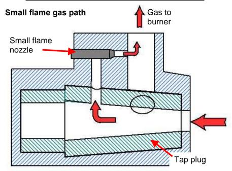
Each burner requires a minimum quantity of gas to ensure stable burning. (If this amount of gas is not supplied, the burner goes out, however when the design delivers excessive gas quantities for the low setting, customers tend to complain that "food is burned".)
