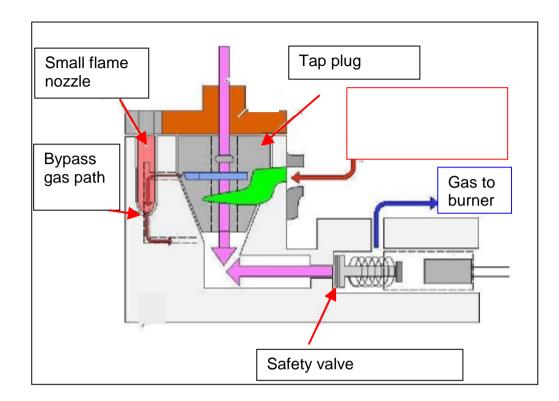
The function of the angle tap with thermal release is basically the same as described above (straight-through gas tap). There are, however, **2 differences:**
