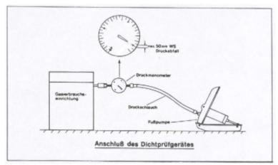
This gas-tightness testing appliance is available under Part Number 340034. It can be connected directly to  $\frac{1}{2}$ " pipe (using 059155 sponge-rubber sealing plug).
