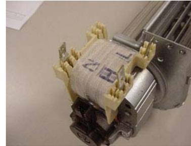
**Figure 18** Tape on cooling fan windings marked to designate terminals
