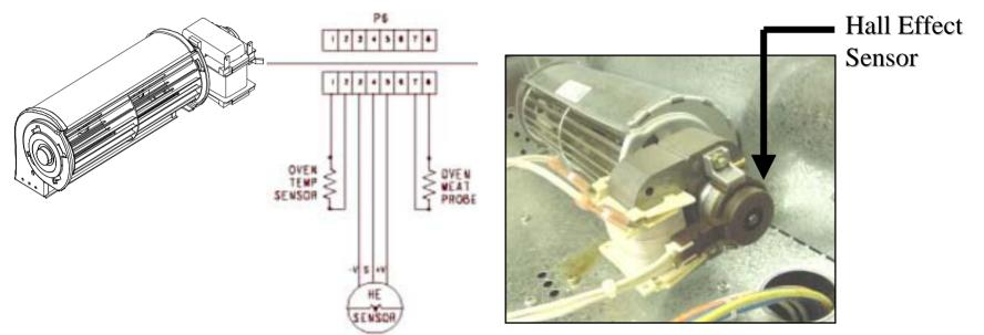
Hall Effect Sensor replaces the air switch as the method of verifying air flow. The sensor is part of the motor assembly and is not supplied as a separate part.
