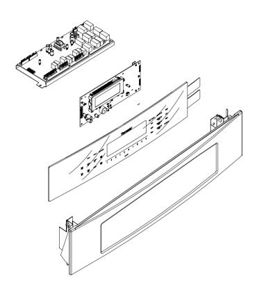
Common Relay Board, Display Head & Touch Sensor Panel used for the "S", "C" & CM series, means reduced inventory and more familiarity with operation.
