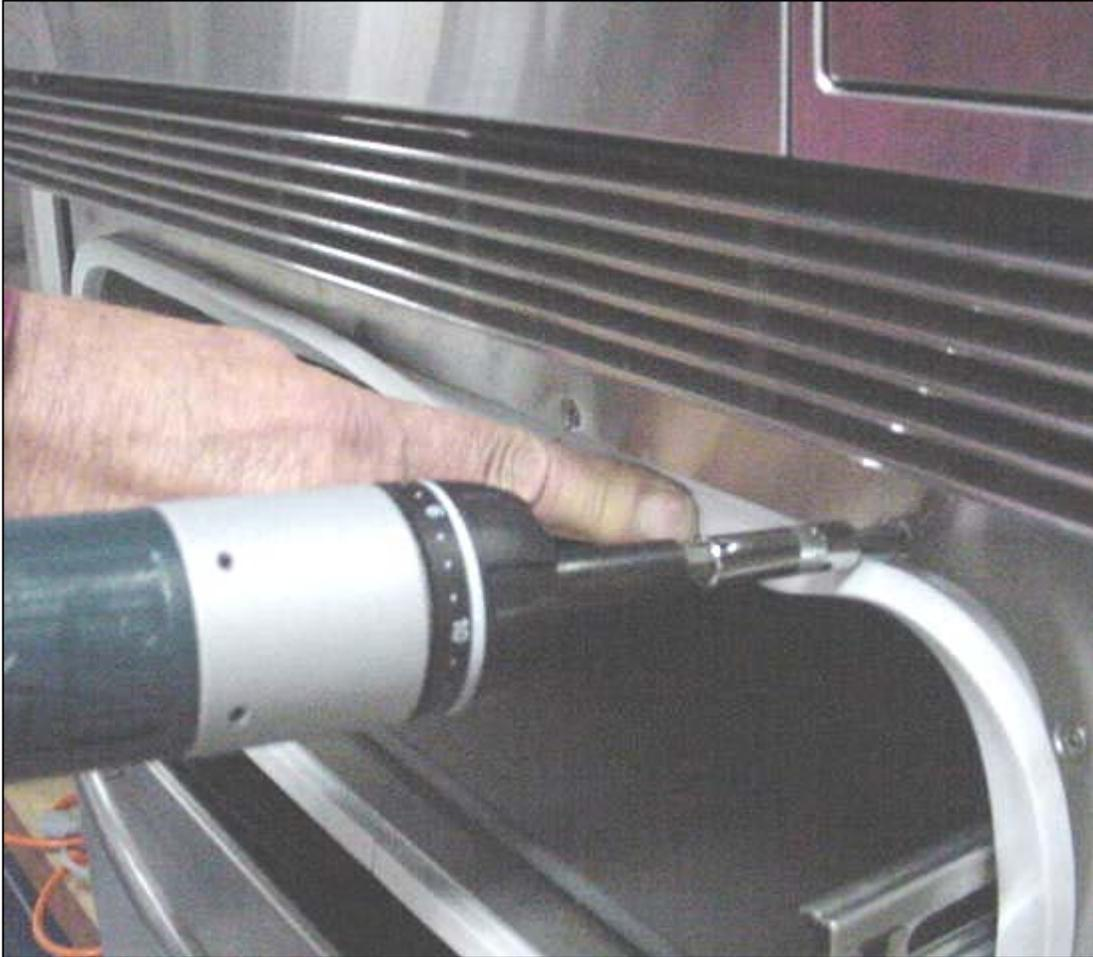
To access controls front frame of warming drawer has to be removed. Peel back drawer gasket and remove the 14 countersunk Phillips screws. Pull off thermostat knob and remove frame
