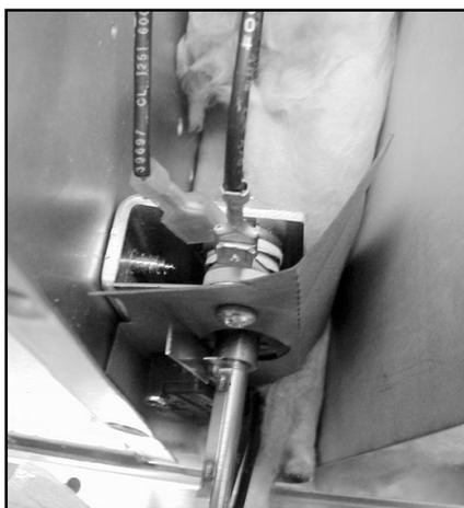
**Piggyback Spade/Terminal** (From On/Off Switch) Placed on terminal closest to shaft (Piggyback facing shaft)
