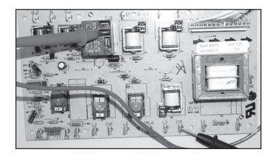
3. Check voltage across the DBL (double line relay) NO output side and the CVL (convection element relay)
