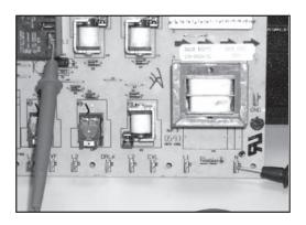
3. Program the unit into a broil cycle. Check voltage across the DBL (double line relay) N.O. output side and BR relay (Broil relay) For 240 Volts. Refer to picture for test points. If you have voltage present go to step 4.
