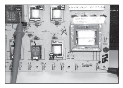
3. Program the unit into a bake cycle. Check voltage across Dbl (double line relay) (N.O. side) to BA relay for 240 volts. Refer to picture for test points. If no voltage replace relay board. If you have 240 volts go to step 4.
