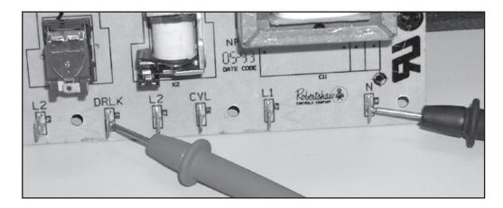
4. If you do not have 120VAC, check for (+ or -) 24V DC at molex connector on the relay board. Pins 1 and 9 on relay board should read 24V DC (+or-); if not then replace the relay board.
