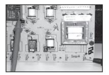
2. Program the unit into Bake or Broil. Check voltage at the DBL (double line relay) com side to neutral. Should read 120 VAC. If no voltage present replace main relay board. If voltage is present then check if cooling fan is running. If cooling fan is not running check wiring and cooling fan motor. If cooling fan is running then check the air switch/sail switch that is mounted to the cooling fan assy. You must remove cooling fan to gain access to air switch/sail switch.
