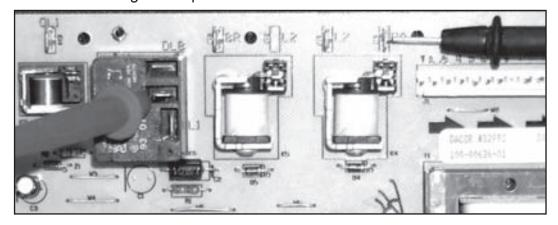
4. Check the HTC (high temp cutout) for open circuit. HTC is a NC switch. The HTC is located by the latch assembly and has a re-settable switch. (see picture)
