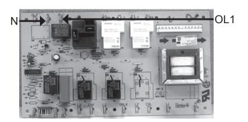
2. Activate the light circuit by pressing the touch pad and listen for the OL1 relay to close then check for 120 volts at OL1. (see picture) if no voltage present replace relay board. If the OL1 (oven light relay 1) doesn't close or you don't hear relay close step 3.
