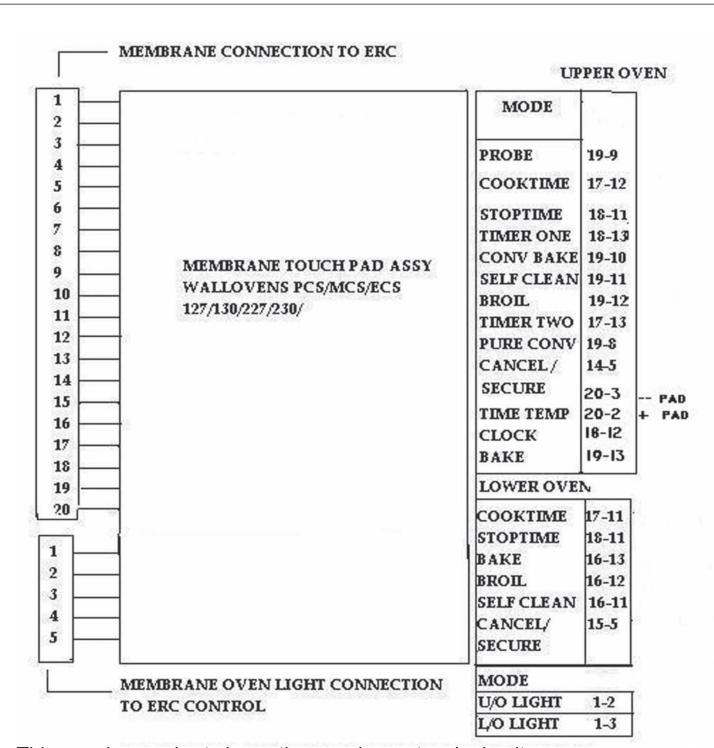
This membrane chart shows the membrane touch circuit.
