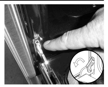
Raise the door so that it is at a 15° angle from the front of the oven. Hold the door with one hand on each side. Lift the door up and out.
