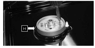
Remove each of the stack burner heads.
