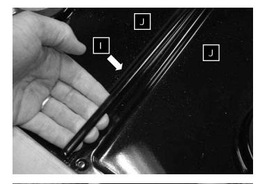
To remove the spill trays, pull up on the back of each spill tray and slip it out of the stainless steel trim piece toward the front of the range. Be careful not to chip the porcelain.
