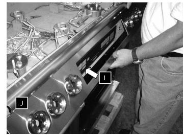
Remove all of the screws that hold the channel support to the cooktop chassis. Lift the channel support out of the chassis.
