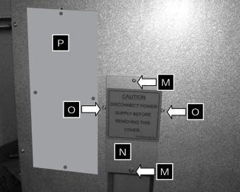
• Remove all of the remaining screws from the back panel and pull it off.
