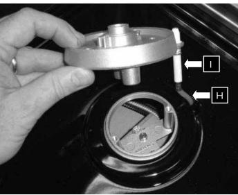
Stack burner igniter replacement
