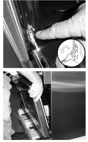
Raise the door so that it is at a 15° angle • from the front of the oven. Hold the door with one hand on each side. Lift the door up and out.
