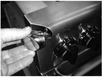
• Remove the side panel screw inside the front panel lip.
