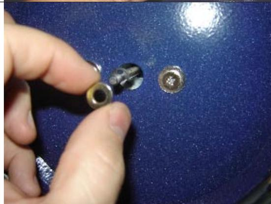
11.7 Remove the 4 screws from the convection motor and remove from the unit.
