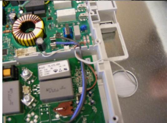
**4.17** View of this white wire that runs under the burner box and is screwed at its Magnetic Core to the front portion of the burner box.
