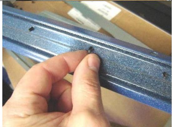
**15.9** Upon installing the mini oven door back together, notice the way that the oven door handle screw spacer has to be installed.
