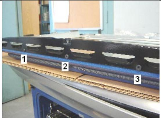
**16.7** The side screw being already removed, remove the 1 screw left on the lower hinge.
