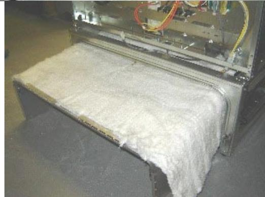
**13.12** Remove the main back cover and remove the hidden bake element wires.
