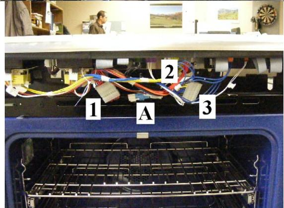
**1.11** Remove the 3 screws that hold the front of the burner box to the center trim.
