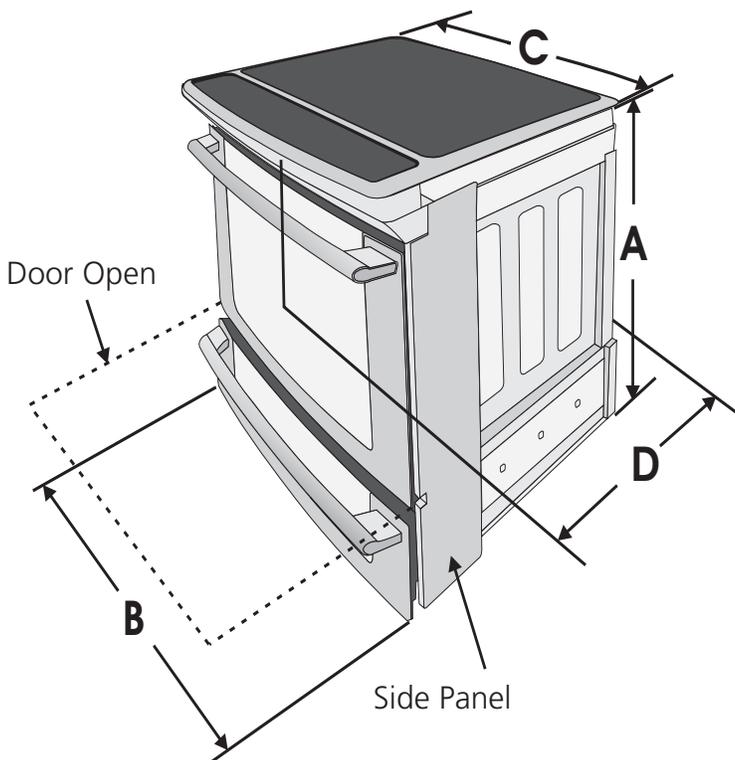
**\*\*\* IMPORTANT:** To avoid cooktop breakage for cutout width (E dimension) of more than 30 1/16" (76,4 cm), make sure the appliance is centered in the counter opening while pushing into it. Raise leveling legs and the rear adjustable wheels at a higher position than the cabinet height (see page 3), insert the appliance in the counter and then level. Make sure the unit is supported by the leveling legs at the front and the wheels at the back and NOT by the cooktop itself.
