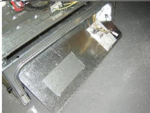
**13.10** Remove the 2 screws (one on each side) that hold the side wall of the mini oven to the bottom brackets.
