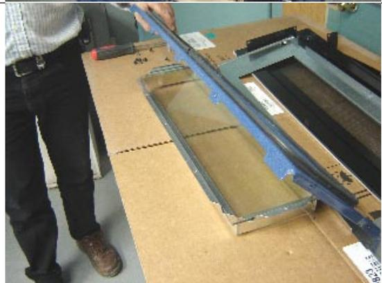
**15.8** Apply pressure (squeeze) on the spring clip of the mini oven door gasket in order to remove it.
