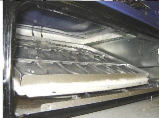
**13 15** Remove the four screws that hold the hidden bake element to its service panel.
