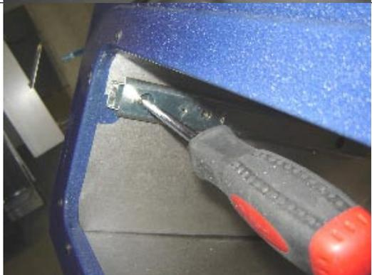
**14.5** Slide the glide out and pull on it in order for the glide to “unlock” from its bracket mounting system.
