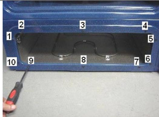
**13.3** Remove the 2 screws that hold the side of the mini oven to the frame of the unit
