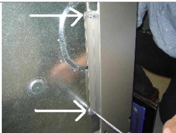
1.6 Pull out the drawer and pull the lower end of this decorative side panel forward, lift the top up and remove from the unit.
