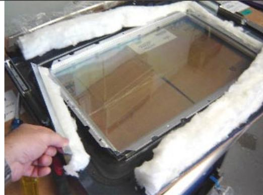
**16.12** Remove the 2<sup>nd</sup> inner glass from the glass pack assembly.
