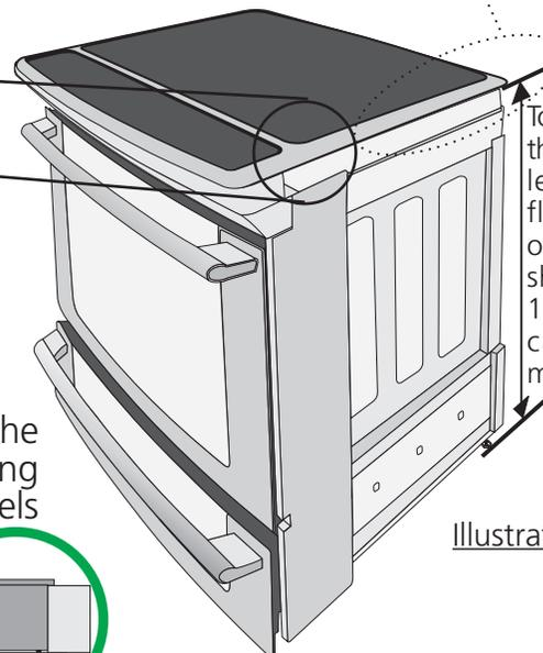
To successfully install the range, the initial level height from floor to underside of cooktop frame should be at least 1/16" taller than cabinet sides as measured in step 2.
