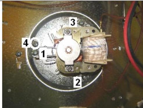
11.8 Remove the rubber washer from the convection shaft.
