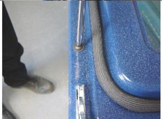
**16.9** Remove the 9 screws that hold the inner door baffle.
