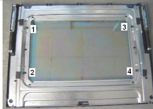
**16.11** Remove the glass holders and insulation.
