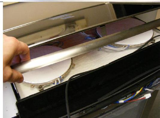
**4.5** Lift the insulation, locate service panel screw and remove it. Remove the service panel.
