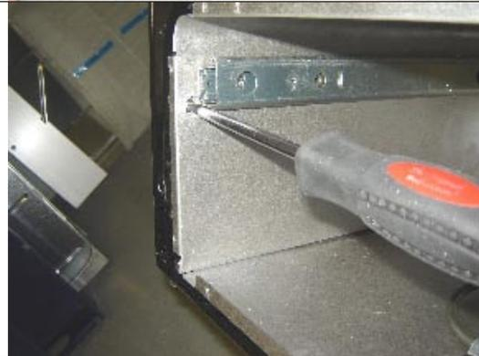
**13.4** Remove the 2 screws from the mini oven bake element
