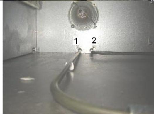
**13.5** Remove the 2 screws (one on each side) of the lower back side of the mini oven.
