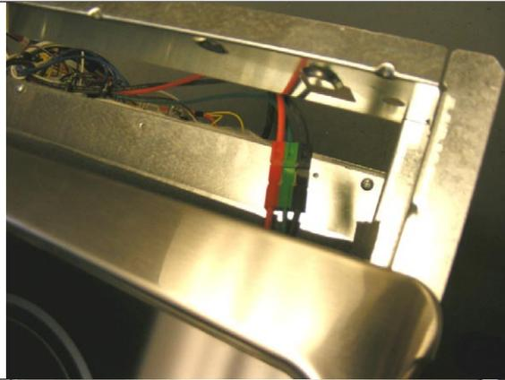
**1.14** Remove the complete burner box and console assembly out of the unit and flip it upside down making sure to protect the customer's table or countertop and for sure, the face of the cooktop.
