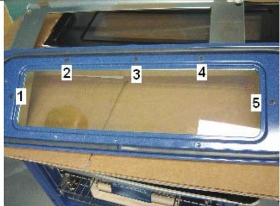
**15.7** Pull the 2 sections apart in order to access the inner door glass and frame.
