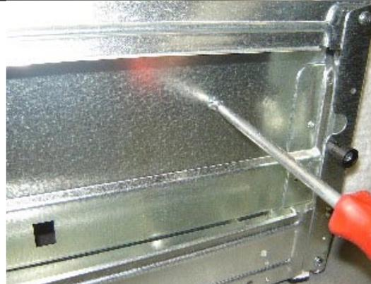
**13.6** Remove the 3 screws from under the back panel of the mini oven.
