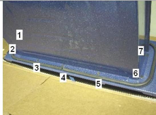
**15.3** Remove the 6 screws from the upper trim, turn the mini oven door and also remove the 6 ones from the lower trim.
