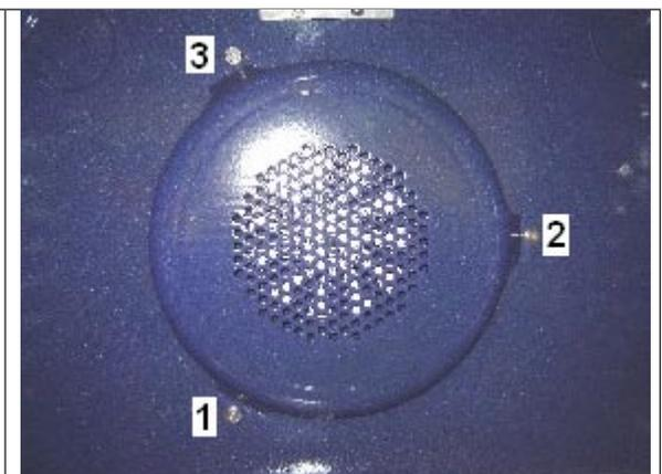
**11.2** Remove the 3 screws which hold the convection element to the back of the oven liner.
