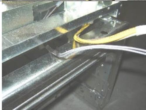
**13.9** Pull the back panel off from the mini oven starting by pulling the lower portion away as shown.
