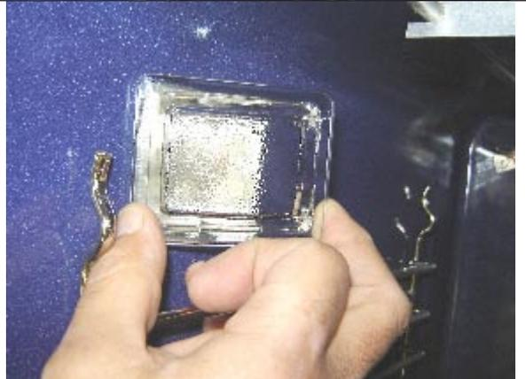
**7.6** Gently pull on the halogen lamp in order to remove it from its socket.
