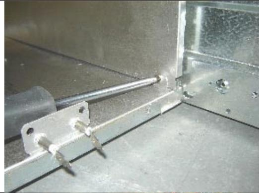
**13.11** Pull the mini oven out from the back of the unit as shown.
