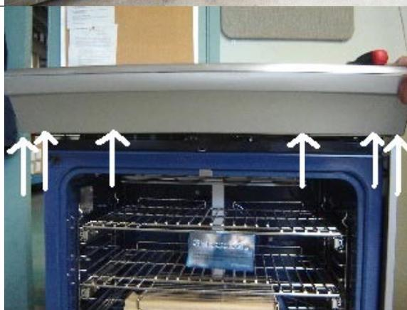
1.8 Gently pull the control panel down and off of the unit.
