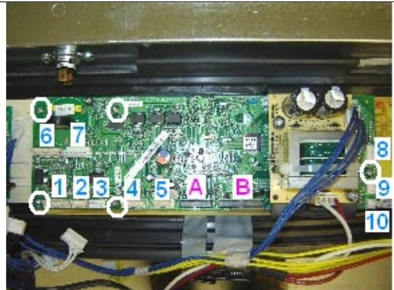
**2.4** Remove the 2 screws that hold the power supply that is over the EOC
