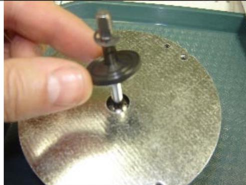
11.9 Properly align the mounting holes from the mounting plate and the convection motor. From the front side of the convection motor...
