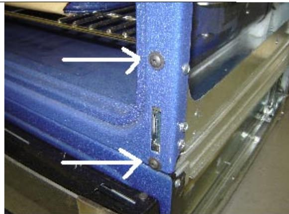
**6.11** Locate hinge receptacle from the side and remove from the back of the front frame
