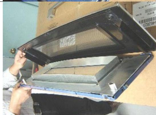
**15.6** Remove the 5 screws that hold the inner mini oven door liner to the inner glass frame assembly.
