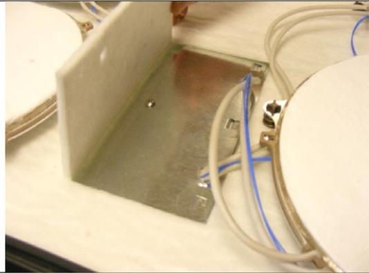
**4.6** Lift the second layer of insulation and unplug the small blue wire then unscrew the 2 large wires.
