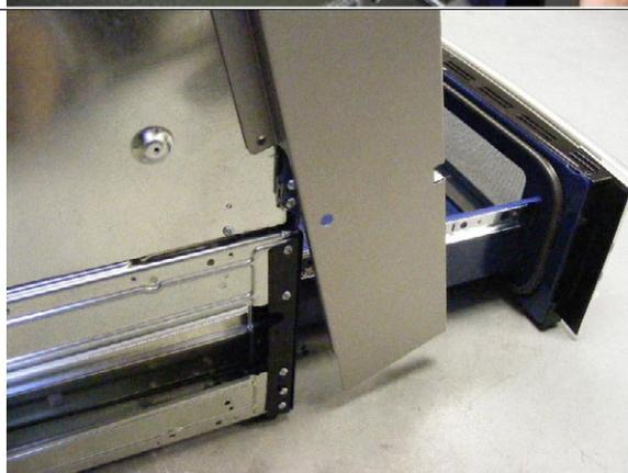
1.7 Remove the 6 screws from the control panel as shown.
