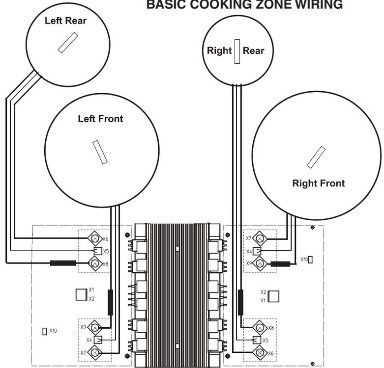
**NOTE:** Connect inductor wire identified by a red sleeve (shortest) to X8 or X9 connectors.
