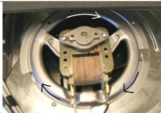
**5.4** When installing the new cooling fan, properly align the 5 circled slotted areas and turn the cooling fan clock wise.
