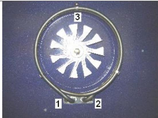
**11.3** Pull the convection element out and unplug the two orange wires.
