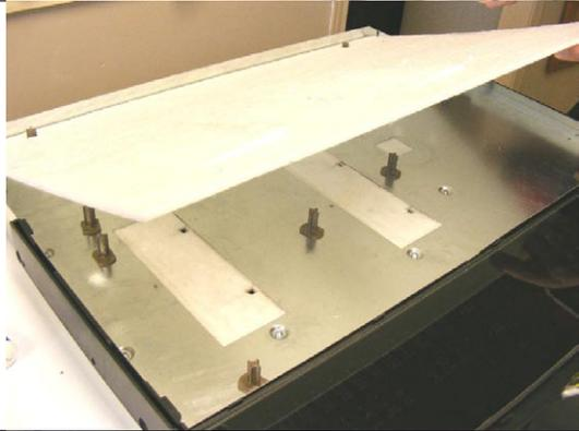
**4.9** Remove the 12 screws (1 to 12) and the one ground wire nut (A).
