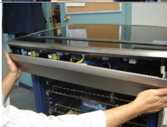
**1.9** Remove the 2 screws that hold the front of the burner box to the upper side panel.
