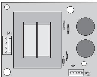
*This board provides power to the electronic control display board.*
