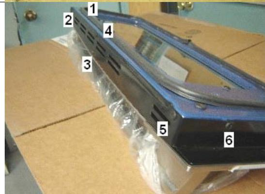
**15.4** Remove the 2 screws which hold the mini oven door handle.
