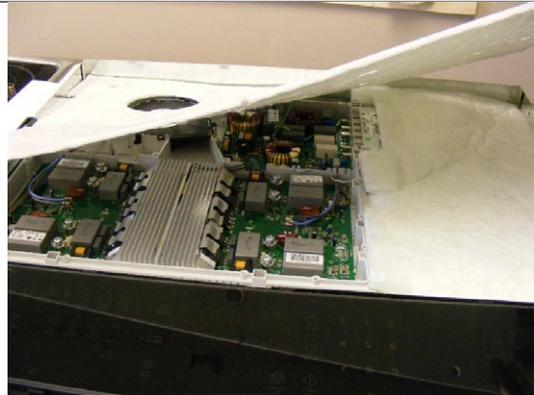
**4.15** Lift and remove the side insulation.
