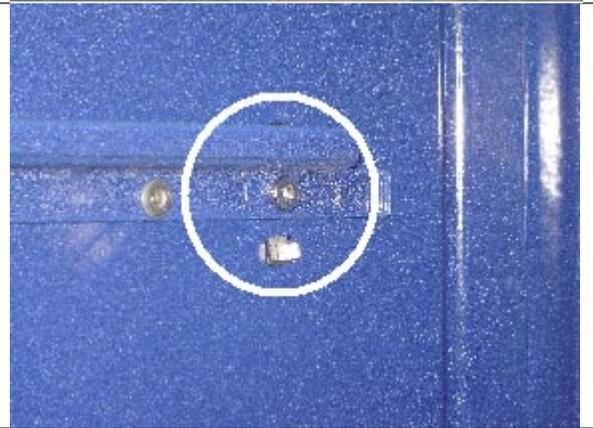
**6.10** Remove the 2 screws which hold the hinge receptacle.
