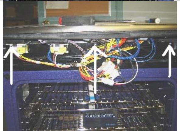
**1.12** Pull the cooktop and console up (at the front) and pull it 6” toward you in order to unlock it from its 2 anchorage point at the back of the burner box.
