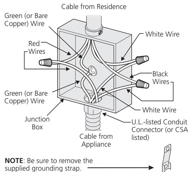
**Figure 6 – 4-Wire Electrical System**
