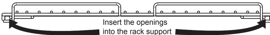
**⚠ WARNING** Always arrange the oven racks when the oven is cool (prior to operating the oven). Always use oven mitts when using the oven.
