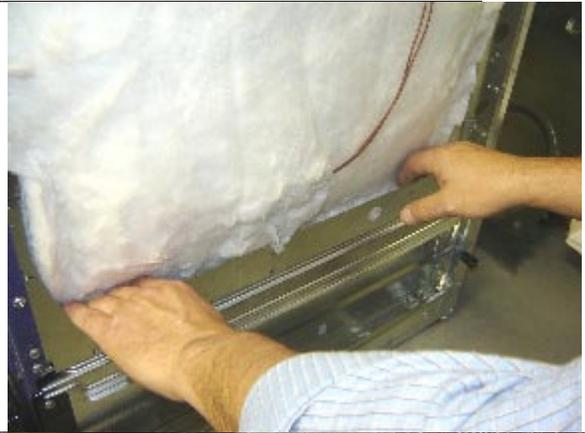
**6.13** Upon replacing the side panel, make sure that it will be inserted between the frame and the upper side panel as shown.
