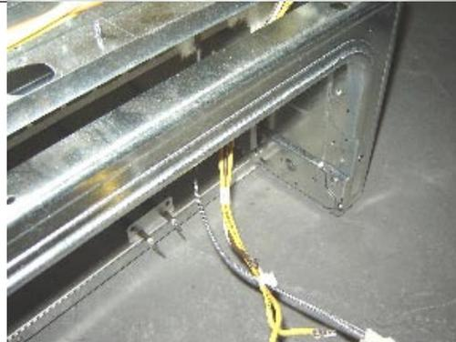
**13.8** Insert these wires between the upper and lower frame as shown.
