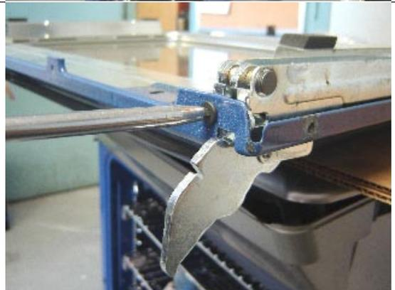
**16.8** Turn the oven door upside down and remove the screw that holds the oven door hinge to the inner door liner.
