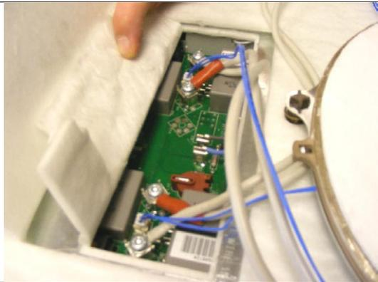
**4.8** Remove the 12 springs, lift and remove the 1<sup>st</sup> layer of insulation.
