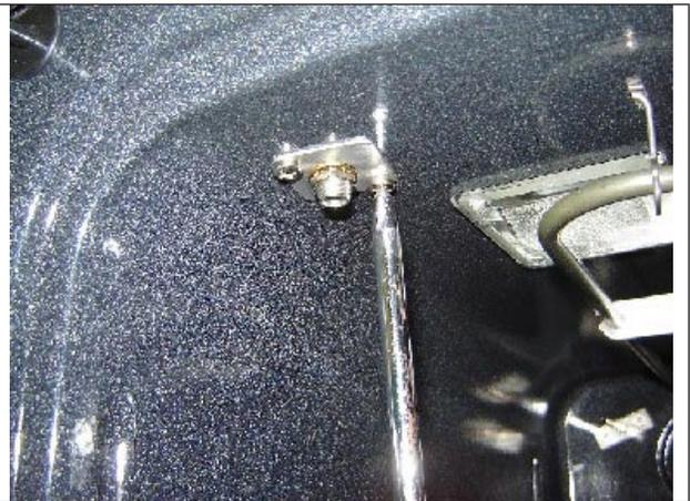
**8.2** Gently pull the meat probe receptacle down and remove the two wires from the meat probe receptacle.
