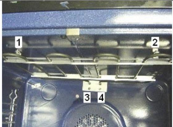
**10.2** Pull the broil element out and unplug the two blue wires.
