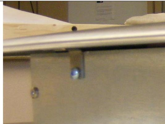
**4.3** Remove the front center screw located under the control panel dead center.
