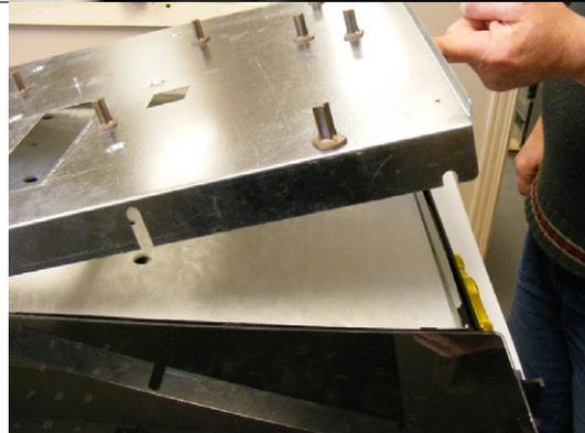
**4.14** Lift and remove the inner insulation.
