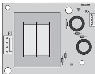
This board provides power to the Electronic Surface Element Control (ESEC).
