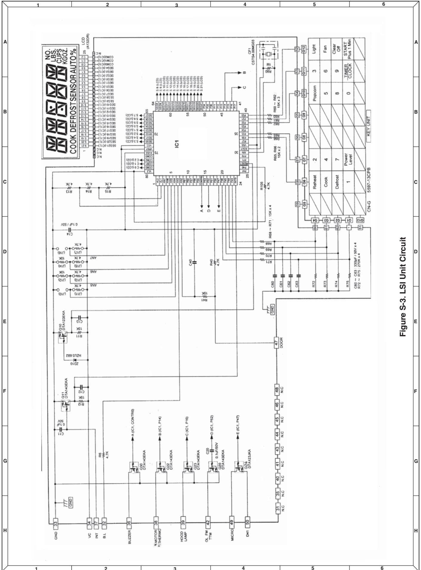
Figure S-3. LSI Unit Circuit
