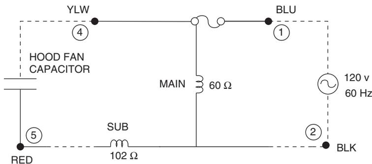
6-PIN CONNECTOR OF HOOD FAN MOTOR
