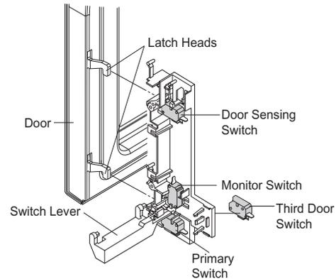
Figure C-1. Latch Switch Adjustments
