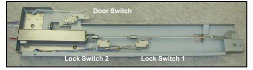
Check wiring continuity and earth insulation back to the power module.
