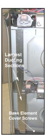
**Note:** When re-inserting element use a wide flat blade or similar object to lift the cavity insulation clear of the replacement element.
