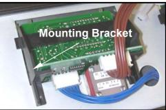
(c) Remove screws securing top and bottom black trims. For V2 models detach black mounting panel by removing retaining screws.
