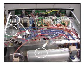
**Note:** TL = Thermal Limiter MTL = Microtemp thermal limiter
