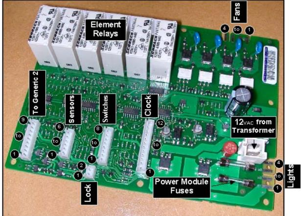
**Note:** This is a Fisher & Paykel specific P.C.B. that drives oven lights, fans, elements and lock motors. It also monitors the sensors and micro-switches and provides power to the control panel.
