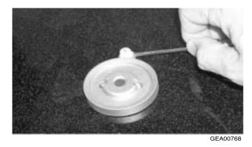
**Caution:** When removing the wire from the igniter, make sure you do **not** damage the heat shrink insulation on the wire. If damaged, repair the wire insulation with fiberglass tape.
