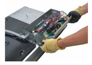
3. Mark and disconnect wiring from the module.
