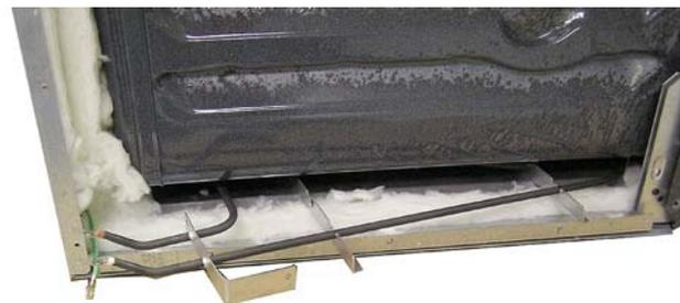
**Note:** Upon reassembly, ensure that the displaced insulation around the oven and its components is returned to its original position.
