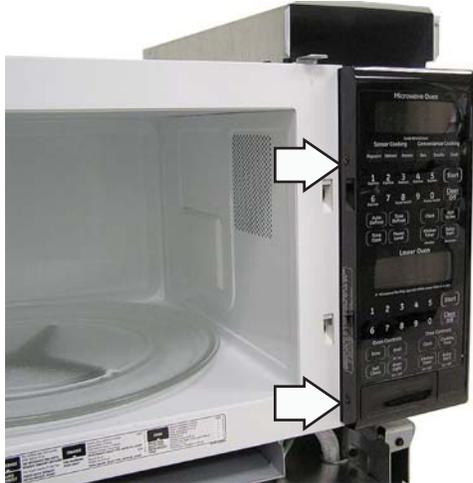
**Note:** There are three tabs on the right side of the control panel assembly. Push the control panel to the left to free it from the housing.
