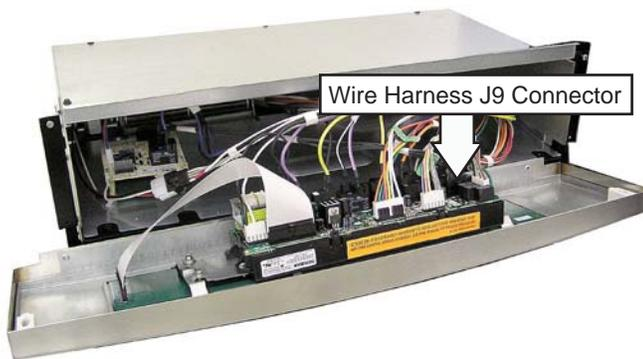
3. Open the oven door and place the control panel on a protected top oven rack.
