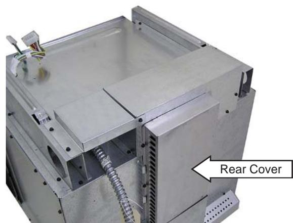
3. Remove four ¼-in. hex-head screws and the duct cover from the oven.
