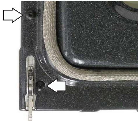
3. Remove the four 1/4-in. hex-head screws that attach the glass and side brackets (glass closest to the outer door glass) to the inner door.
